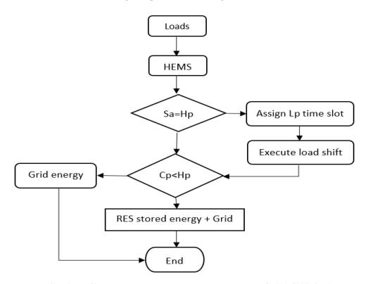
**Figure 1.** Flowchart of home energy management systems. Sa = Specified shiftable loads, Hp = High peak hours, Cp = Current energy price, Lp = Low peak hours.
