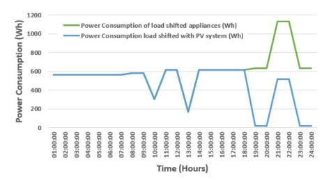
**Figure 12.** The 24-h winter power consumption profile for load shifted appliance with and without a PV system.
