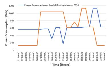
Figure 11. 24-h winter power consumption graph for load shifted with and without an HEMS.
