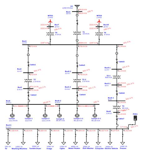
Figure 9. Simulation results of model presented in Figure 5.
