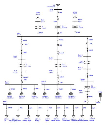
Figure 5. HEMS and mixed RESs (solar and wind).
