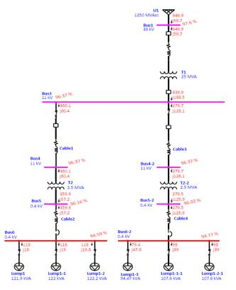
Figure 6. Load flow simulation results of model presented in Figure 2.
