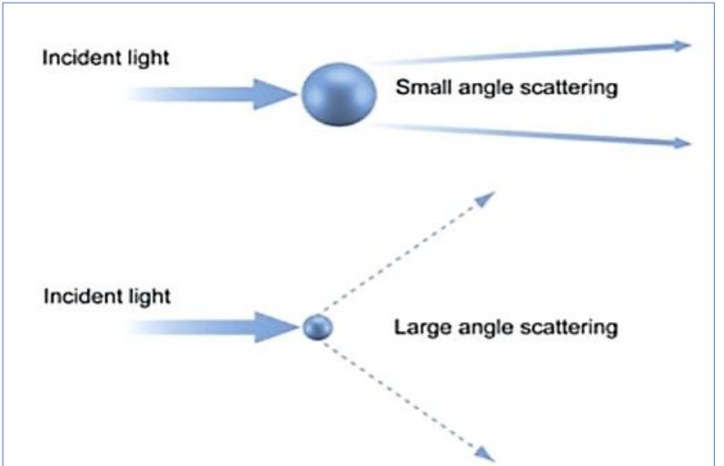
Grain sizing was calculated by directing a laser beam at the sediment particulate. The measured intensity of angular disparity in scattered light is used to calculate grain size
