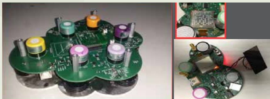
Figure 2. 3D view of SERENO (PCB top view) where the 6 (version 1, left side) or 4 (version 2, right side) gas sensors are shown. Version 2 features a local display.
