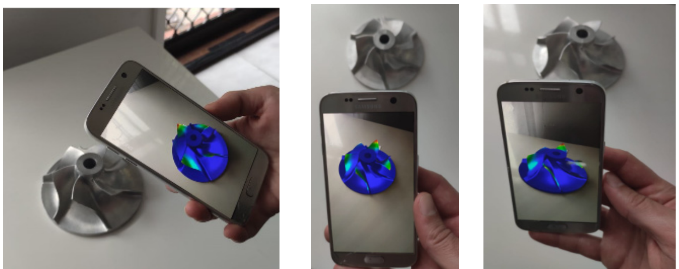
Figure 8. Modal analysis simulation results on the mobile AR visualization.
