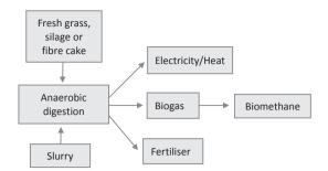
Figure 2 Overview of energy production from pasture, or from pasture-based biorefinery products, via anaerobic digestion. Combining energy production with higher value animal feed additives (Figure 1) can create additional value.
