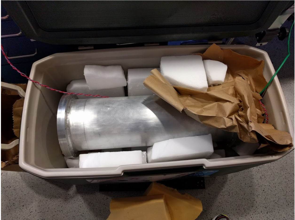
Figure 4.13: Thermal testing the pressure vessel using dry ice
