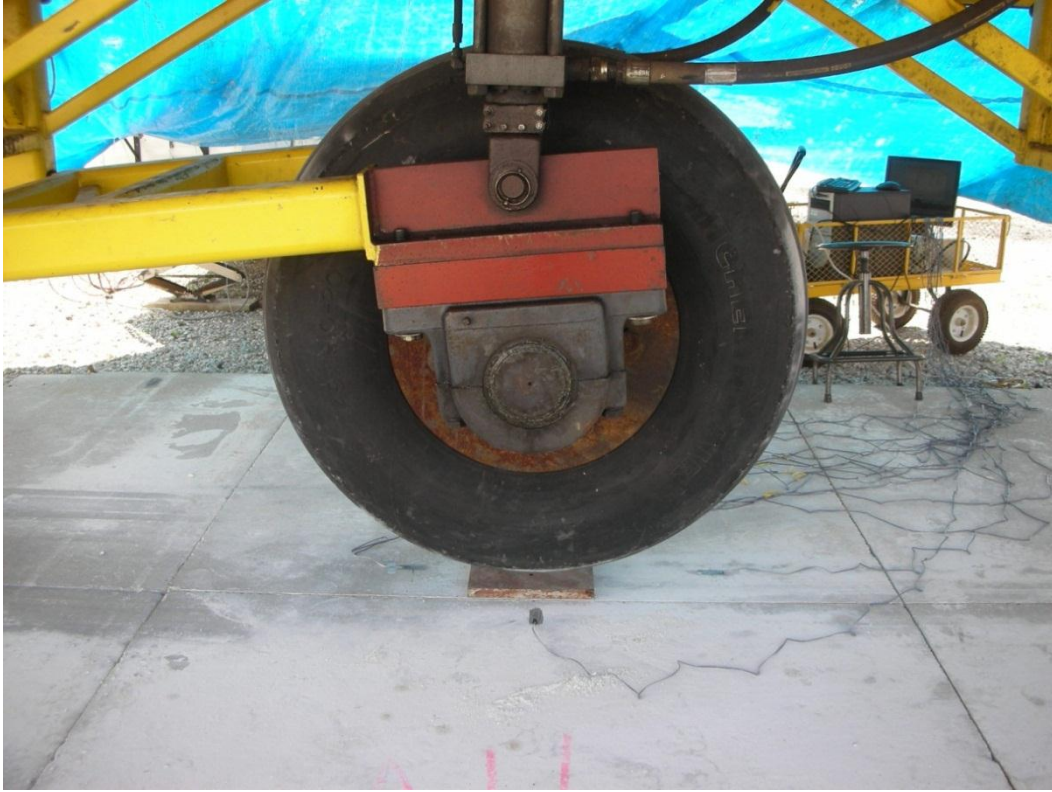
Figure 3.4 ATLAS tire used for static loading of in-situ pavement during initial configuration
