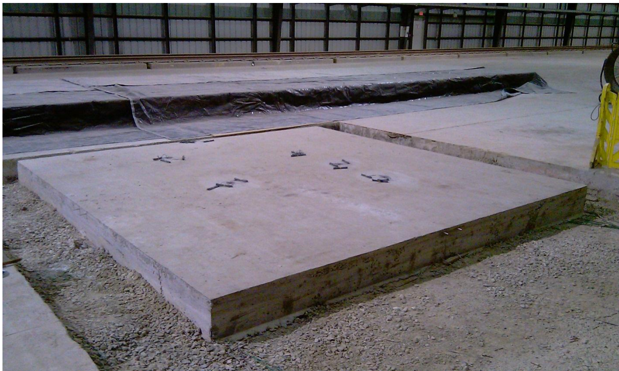
Figure 4.20 Overview of six strain rosettes attached to 15' squared slab
