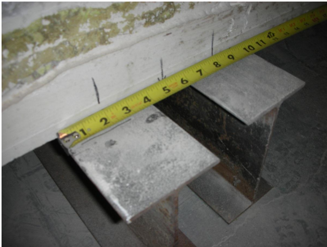
Figure 2.3 Close-up view of centrally supported slab, the 2 inch span and flange supports
