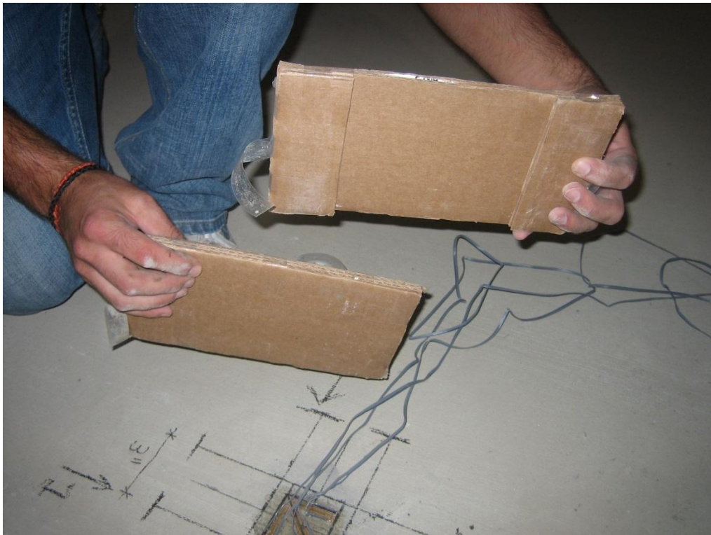
Figure 4.35 Cardboard guides used to protect gages during saw passes
