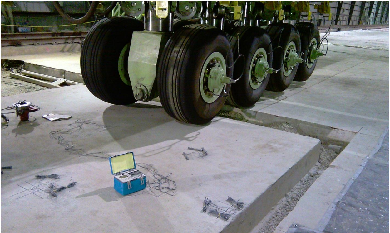
Figure 4.28 Wheel loads positioned along center-edge for test C1
