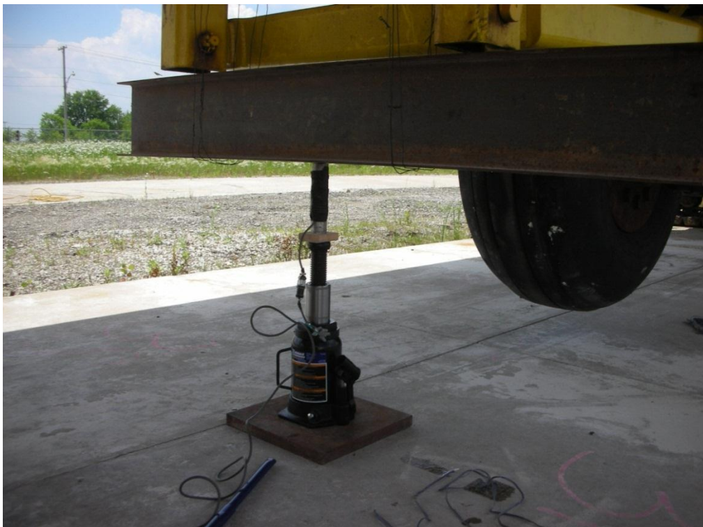
Figure 3.3 Bottlejack using ATLAS wheel carriage as reaction frame, load cell and steel beam for flush surface
