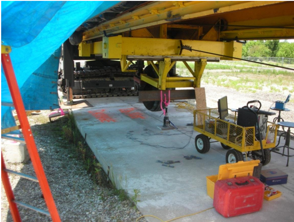
Figure 3.2 View of slabs, ATLAS wheel carriage, bottlejack, tarp to shade from sunlight and miscellaneous testing equipment
