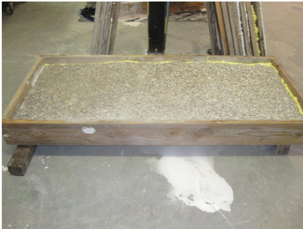
Figure 2.1 Slab flipped exposing its underside. Form fitted at its edges in preparation for Hydrocal plaster
