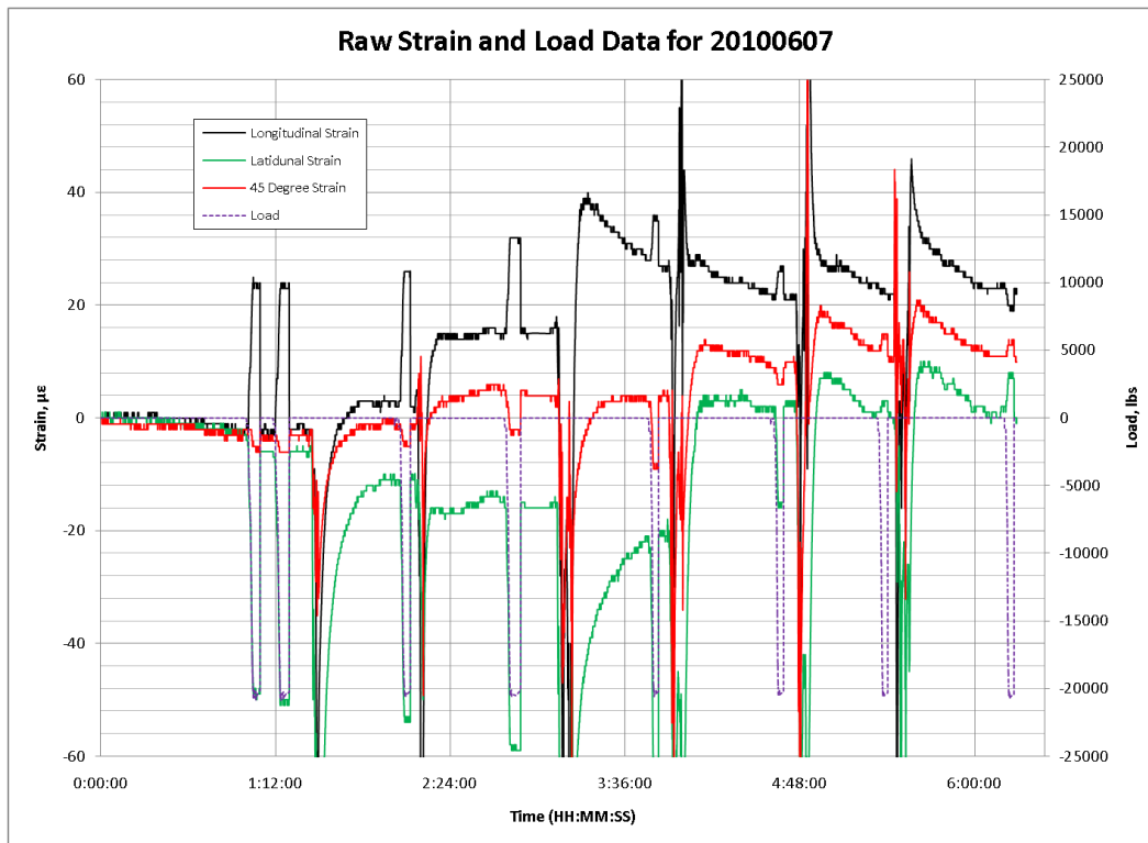
Figure 3.13 Strain and load data for Slab 2S where the strain rosette is spaced 2 feet from applied load and isolated with notches spaced 3 inches apart
