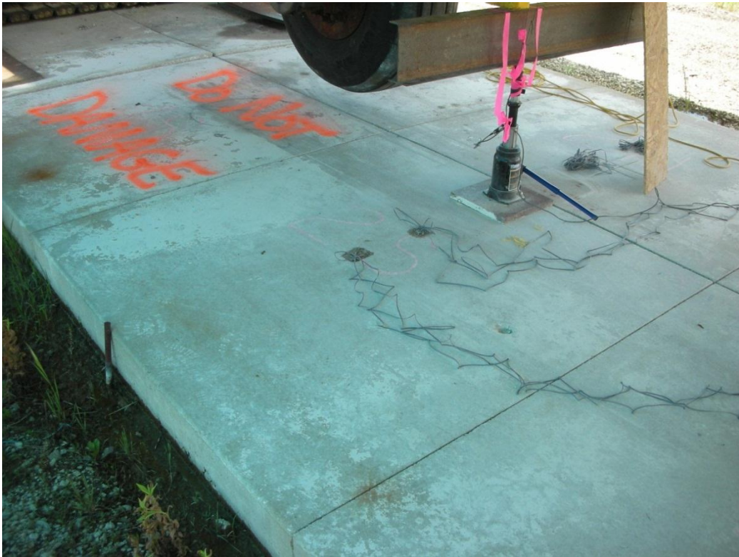
Figure 3.5 Strain rosettes spaced either 2 feet or 3 feet from applied load
