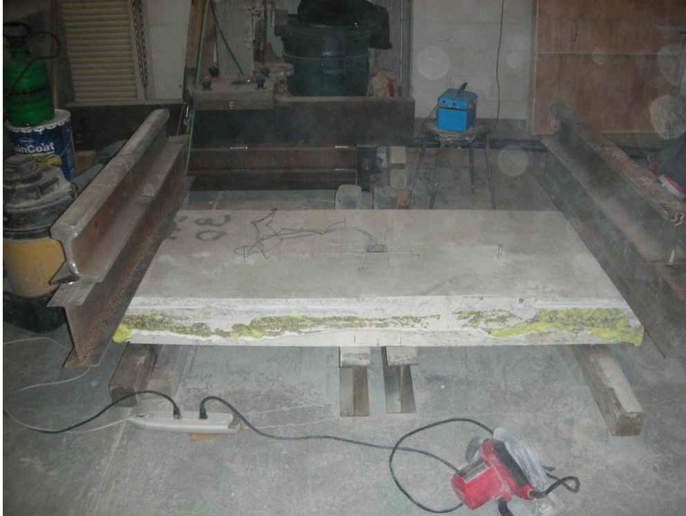
Figure 2.2 Centrally supported concrete slab with 220 lb edge loads applied to produce tension along the top surface
