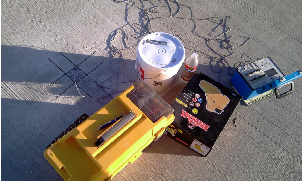
Figure 5.23 Testing at ORD Fuel Depot with bucket providing shade to testing location.
