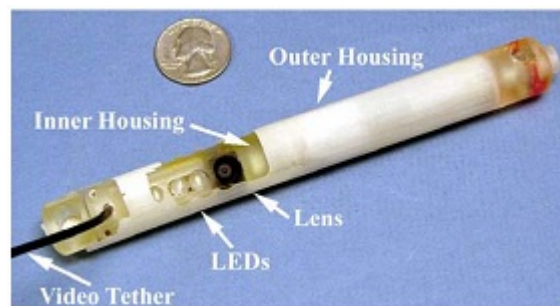
Figure 2.5: (a) Schematic of Ceiling Camera Robot with Magnetic Handle and (b) Photograph of Robot [36] (© 2009 IEEE)
