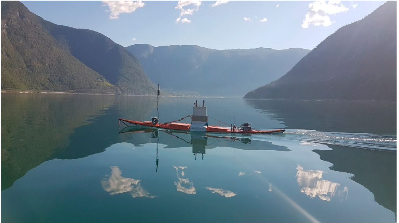
Figure 5.1 Kayakdrone surveying sprat in Sognefjord.
