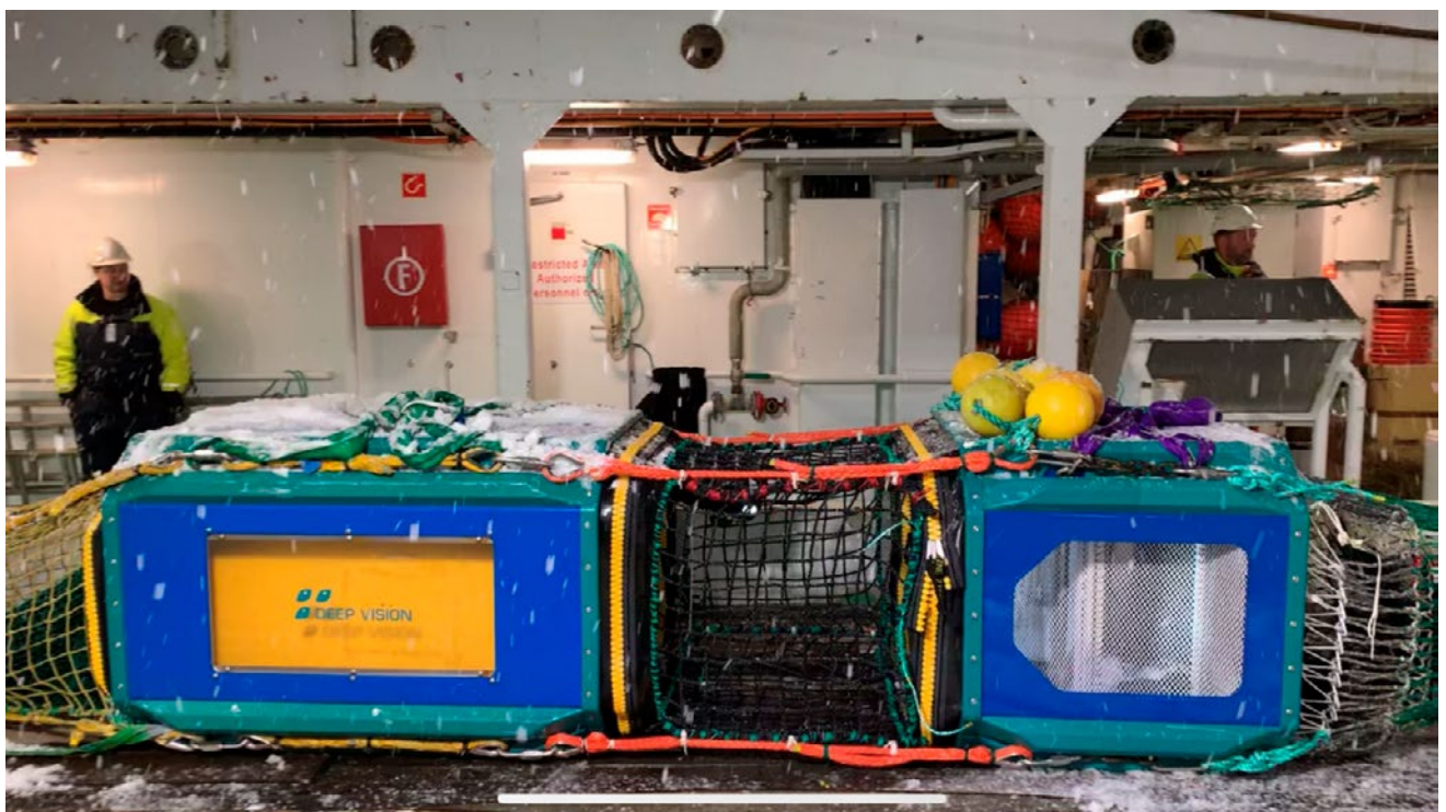
Figure 3.1 The Deep Vision (left) and the ASM (right) mounted to the VITO pelagic trawl.
