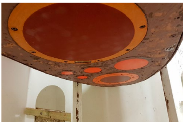
Fig. 6.1 The ES150-3C transducer and transceiver mounted in the front part of the drop keel of G.O.Sars, inside a ES38B transducer adapter ring.
