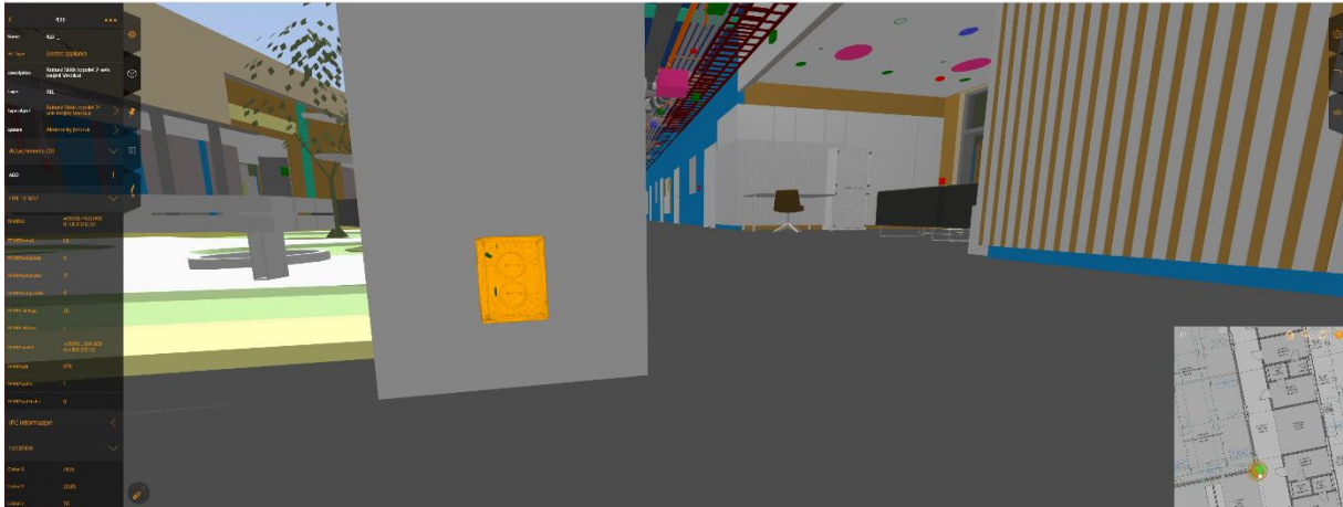
Figure 6.3-1: Digital illustration of electricity details at NPK where other ‘irrelevant’ technical installations have been filtered away. An outlet is highlighted in orange, with all accompanying information displayed to the left (image courtesy of Skanska).
