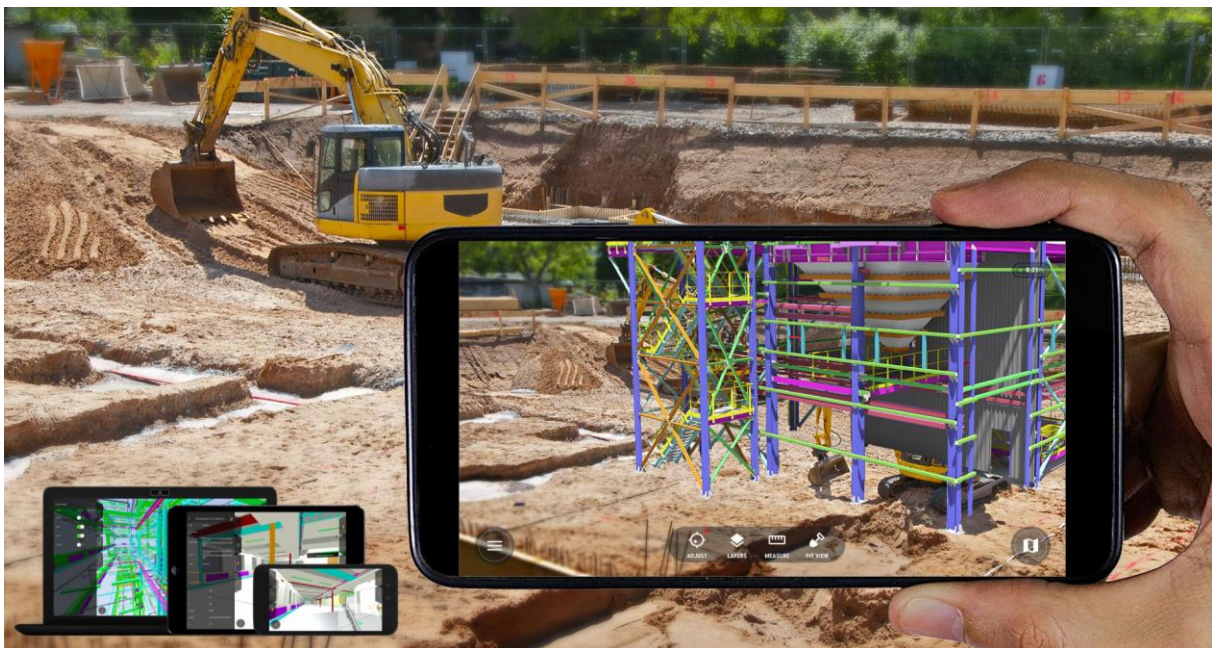
Figure 3.3-2: Illustration of BIM interface through tablets and smartphones (vGIS, 2021).
