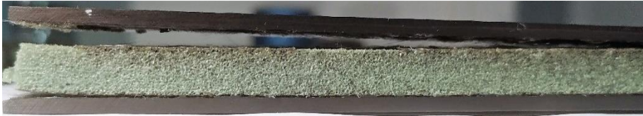
Figure 2.18- Debonding of the core facing interface
