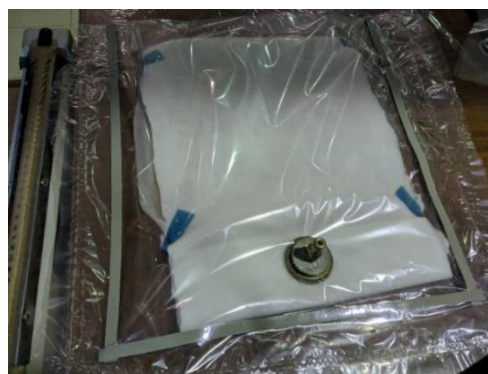
Figure 3.3- Vacuum bag with CFRP 12-layer unidirectional board before the curing prosses
