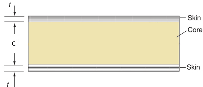
Figure 2.10- Sandwich beam (adapted from [27])
