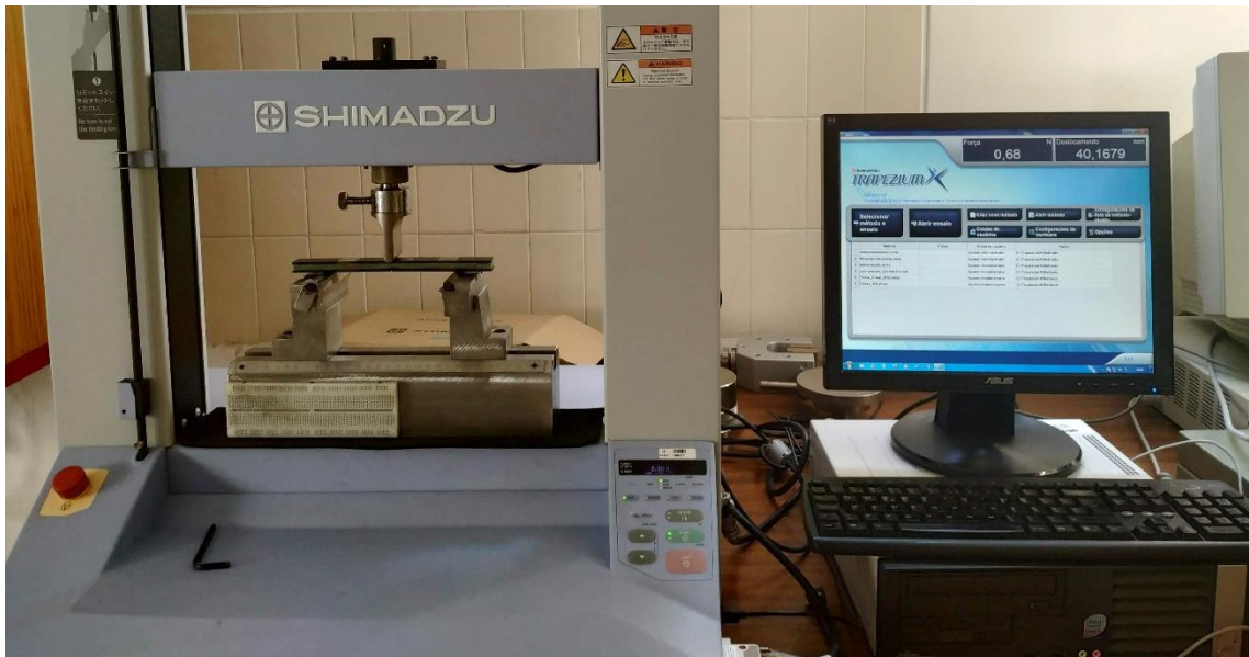
Figure 3.9- Flexural tests experimental setup
