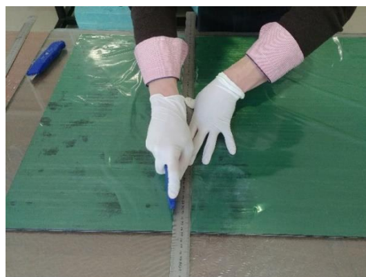
Figure 3.1- Prepreg transverse cutting
