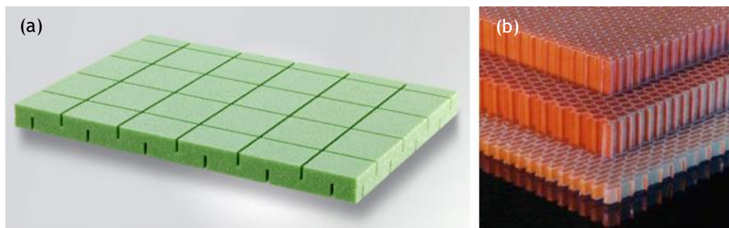
Figure 2.11- a- AIREX® C70 foam core [30], b- Aramid (Nomex®) honeycomb cores [31]
