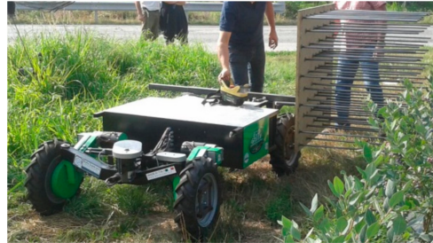
Figure 1. Prototype machine for blueberry harvesting.
