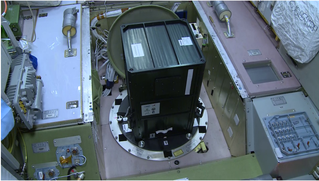
Figure 13. Mini-EUSO mounted on the UV transparent window of the Zvezda module. The velocity vector is usually toward the bottom of the picture, in the side marked as '1'.
