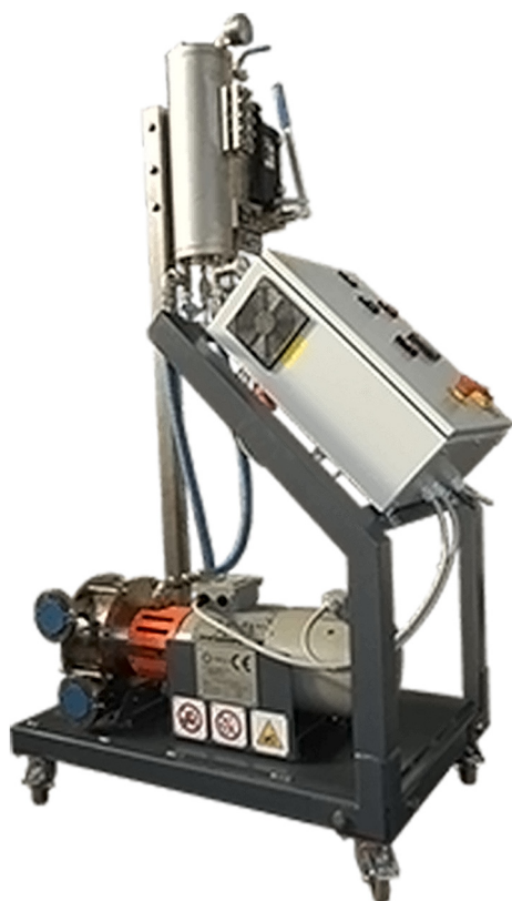
Fig. 3. Rotor-stator generator of HC (E-PIC S.r.L.) from the authors' laboratory.
