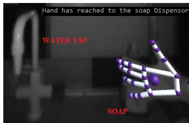
Figure 4.4.1: The presence of a hand on the soap is detected with the Leap sensor The python script is added in the appendix section of the document.
