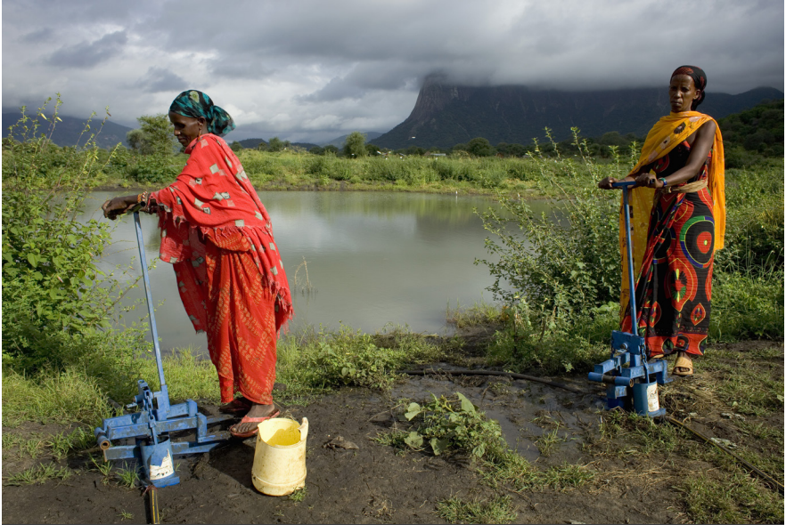
Water is pumped from the pan using a treadle pump. JilloDabassa (on left) is just one of the community members who will take their turn to pump water for the benefit of all. The water is carried to water tanks which then gravity feed the irrigation pipes.
