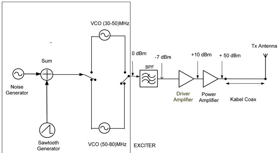
**Gambar 2. Diagram blok Radio Jammer**
