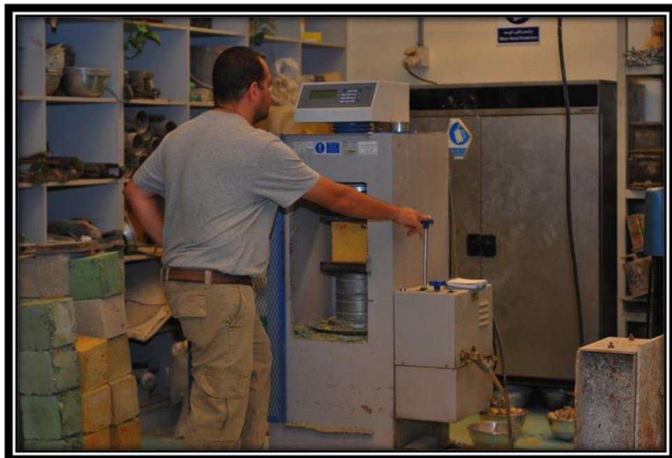
Figure 3.3 Compressive Strength Testing
