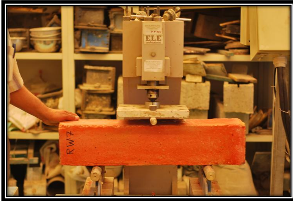
Figure 3.4 Flexural Strength Testing
