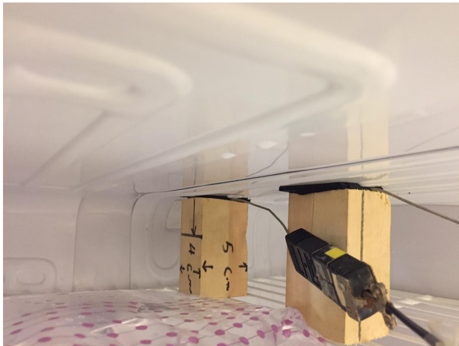
Figure 3.9: Evaporator inlet and outlet thermocouples attachment.
