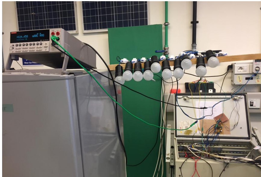
Figure 3.27: Current transducer calibration setup.
