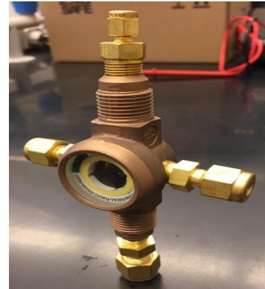
Figure 3.23: Sight glass with thread drills and with the connections tightened in it.
