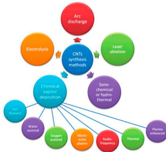
Figure 1.10: The currently used methods for fabricating CNTs [41].
