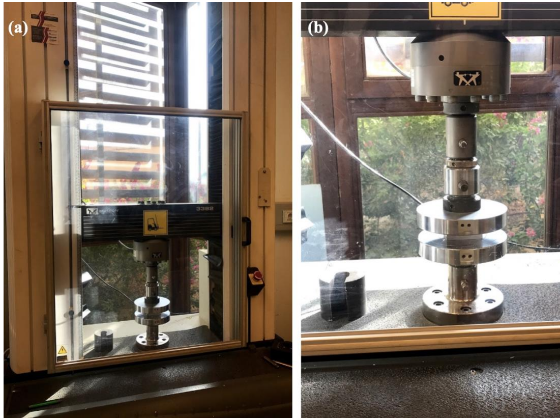
Figure 3.7: A universal testing machine used for compacting CNT samples. The image was taken at AUC materials testing lab.
