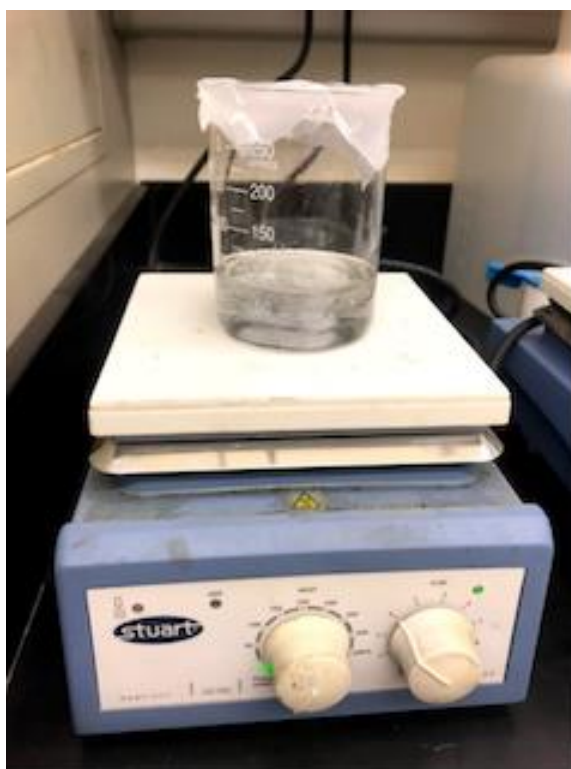
Figure 3.2: The magnetic stirrer used for sample dispersion; image was taken at AUC chemistry lab.
