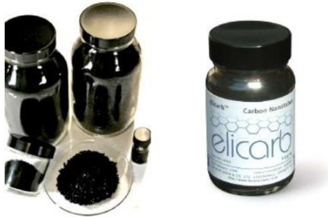
Figure 3.1: As received dry powder form of Elicarb MWCNTs supplied by Thomas Swan [83].
