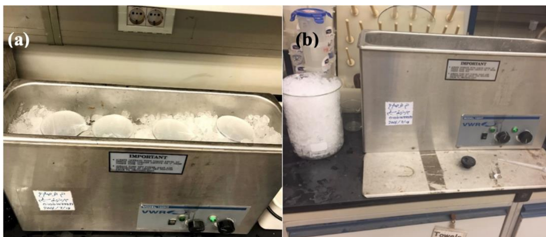
Figure 3.3: The sonication process. (a) The sonication bath after placing the two samples was divided into four beakers and (b) The sonication bath prior to placing the ice and the samples. The images were taken at AUC chemistry research lab.
