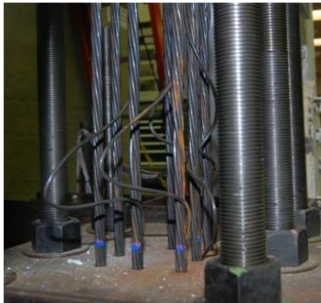
Figure 5.27 Photograph of Specimen A4 Unraveled Post-Tensioning Strands After Single Wire Fractures
