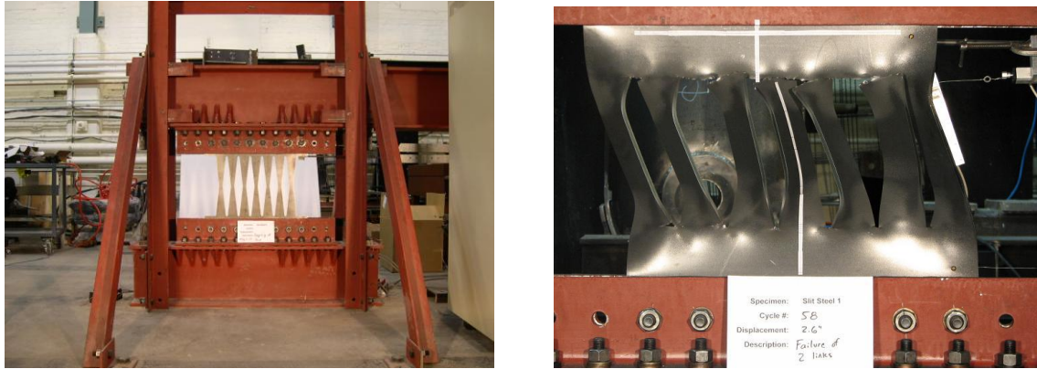
Figure 2.15 Fuse Test Setup (Left) and Fractured Slit Plate Fuse (Right) (from [Ma et al. 2010c])
