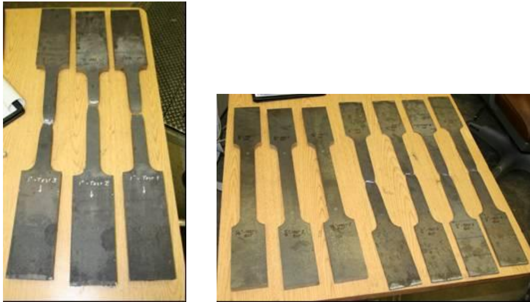
Figure 4.15 Tension Coupons for 25.4 mm (1") Thick (left), 15.9 mm (5/8") Thick (middle), and 6.4 mm (1/4") Thick Fuses (right)
