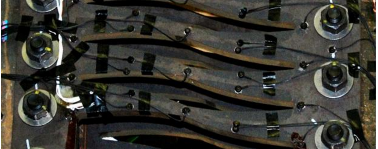
Figure 8.16 Photograph of Specimen A4 Fuse Showing Plasticity in the Links
