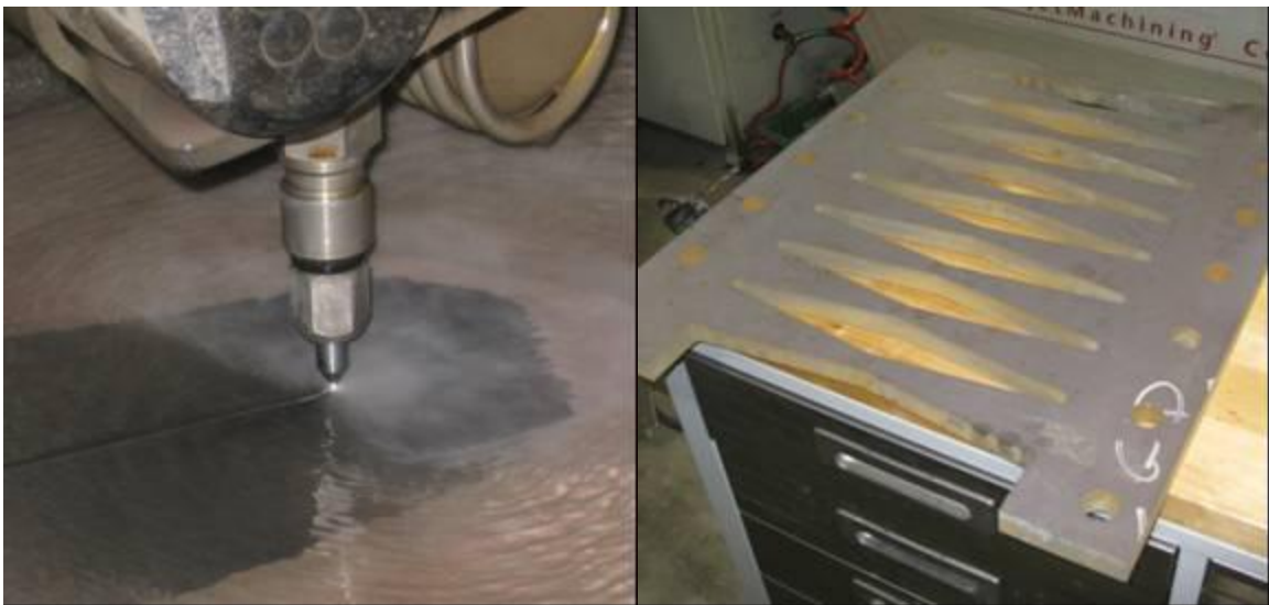
Figure 4.12 Photo of Water Cutting (Left) and Finished Fuse (Right)
