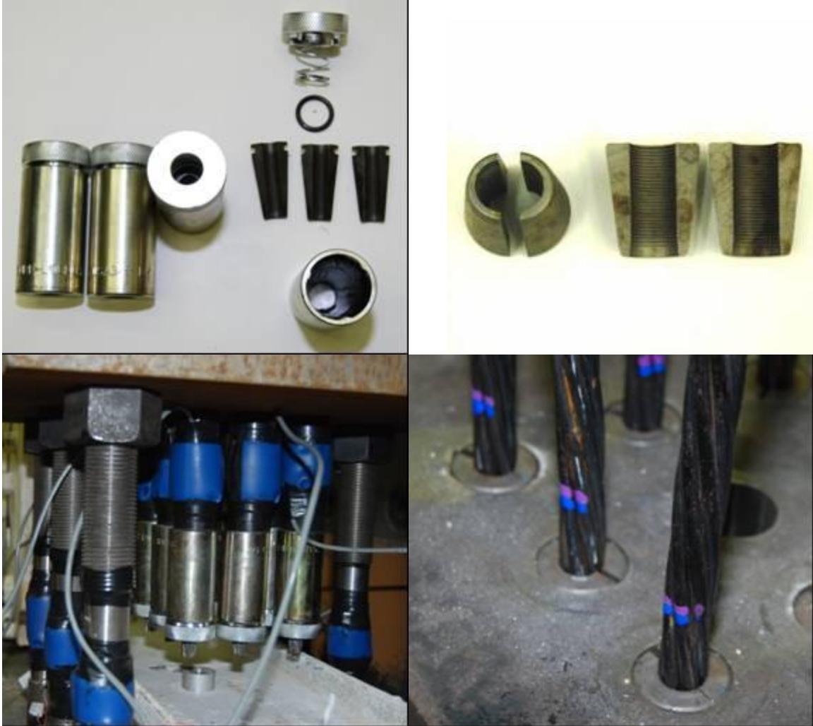
Figure 4.9 Post-Tension Chucks (top left), Wedges (top right), Installed Chucks (bottom left), and Installed Wedges (bottom right)
