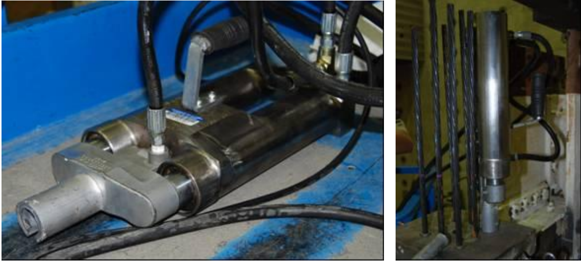
Figure 4.17 Post-Tensioning Jack (left), and Post-Tensioning in Progress (right)
