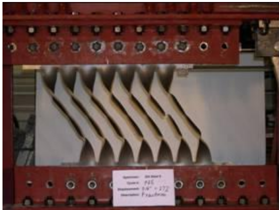
Figure 2.17 Picture of Stanford University Fuse Test B56-09 (left), and the Resulting Load-Deformation Response (right)
