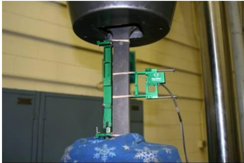
Figure 4.16 Photograph of the Fuse Material Tension Test
