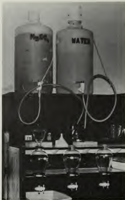
Fig. 5.—Laboratory arrangement for the final separation of corn rootworm eggs from soil. Magnesium sulphate and water flow by gravity into the separatory funnels. The funnels can be removed from the stand.
