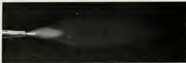
Fig. 2.—This flame is variously called an excess acetylene, a reducing, or a carburizing flame
