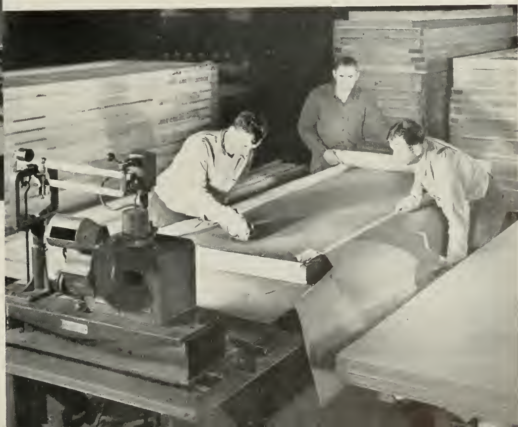
Fig. 12. (Left). Hydraulic stretcher leveling machine, Wood Works. In this machine the stainless steel sheet is stretched just enough to produce a smooth and even surface.
