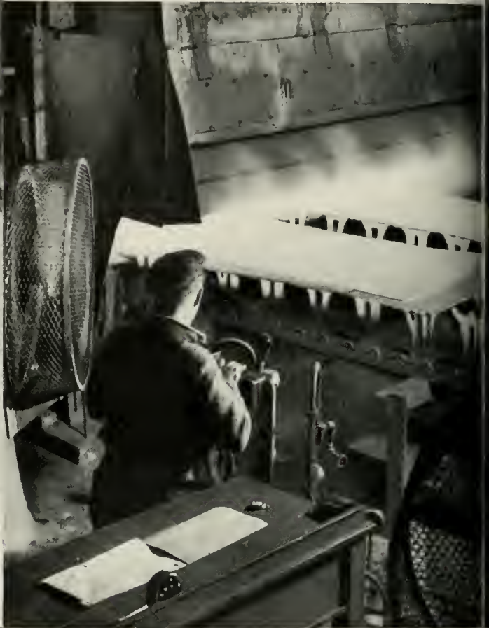
Fig. 7. (Below). Continuous annealing furnace, Wood Works Carnegie-Illinois, in which stainless steel sheets are heat treated. The stainless sheet is laid on a "rider" or "waster" sheet for its ride through the furnace. The conveying mechanism is below the furnace except for the dogs (supports projecting from a continuous chain belt) which hold the sheets. The dogs project through slots in the furnace bottom. Note the two ventilating fans which help to keep the operator comfortable.
