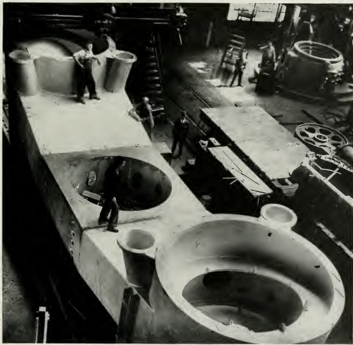
South Cross Member of 200-inch Telescope. (See page 6)
