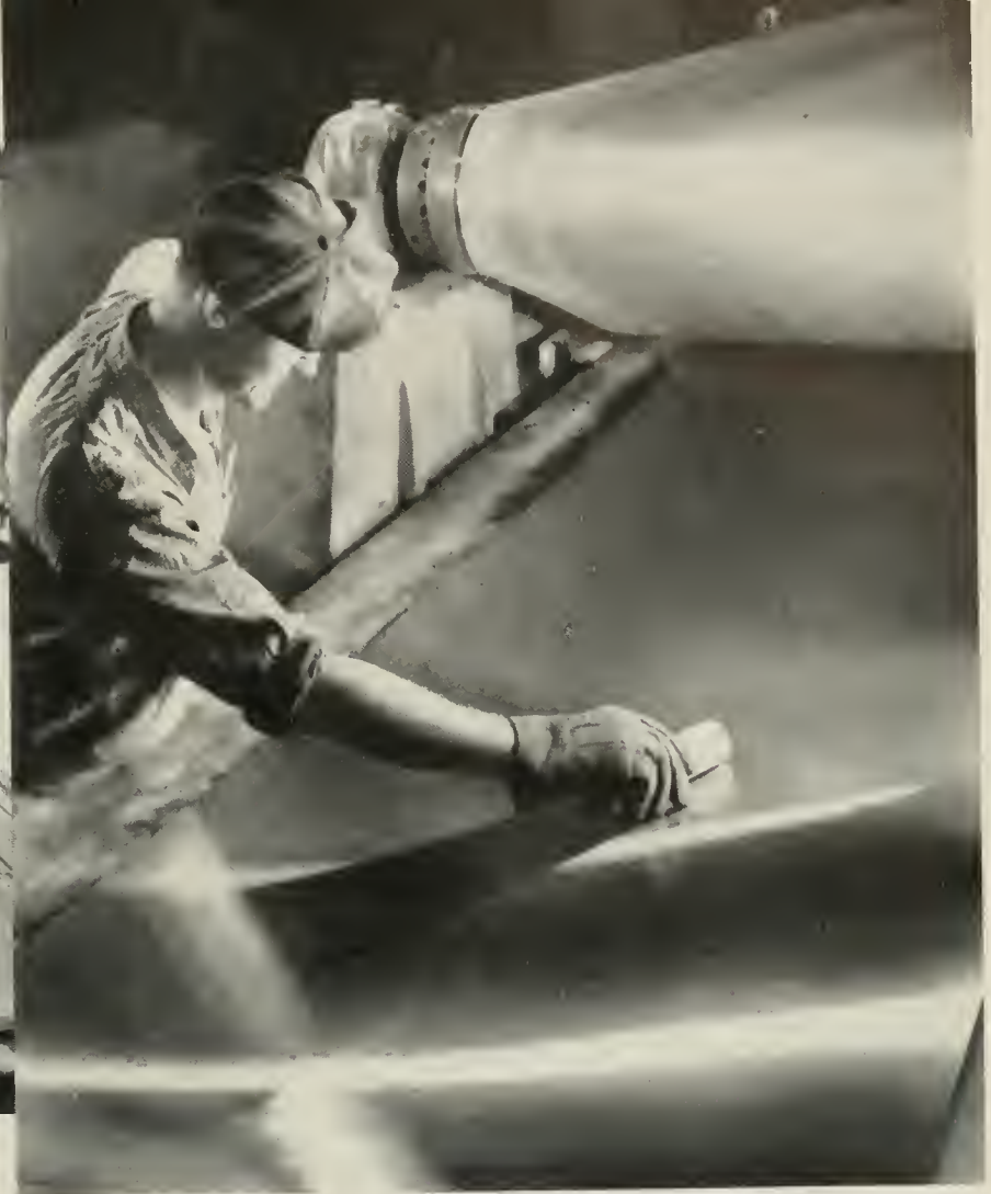
Fig. 10. (Upper left). Rough-grinding stainless steel, Wood Works. The operator is slushing grease on the sheet.
