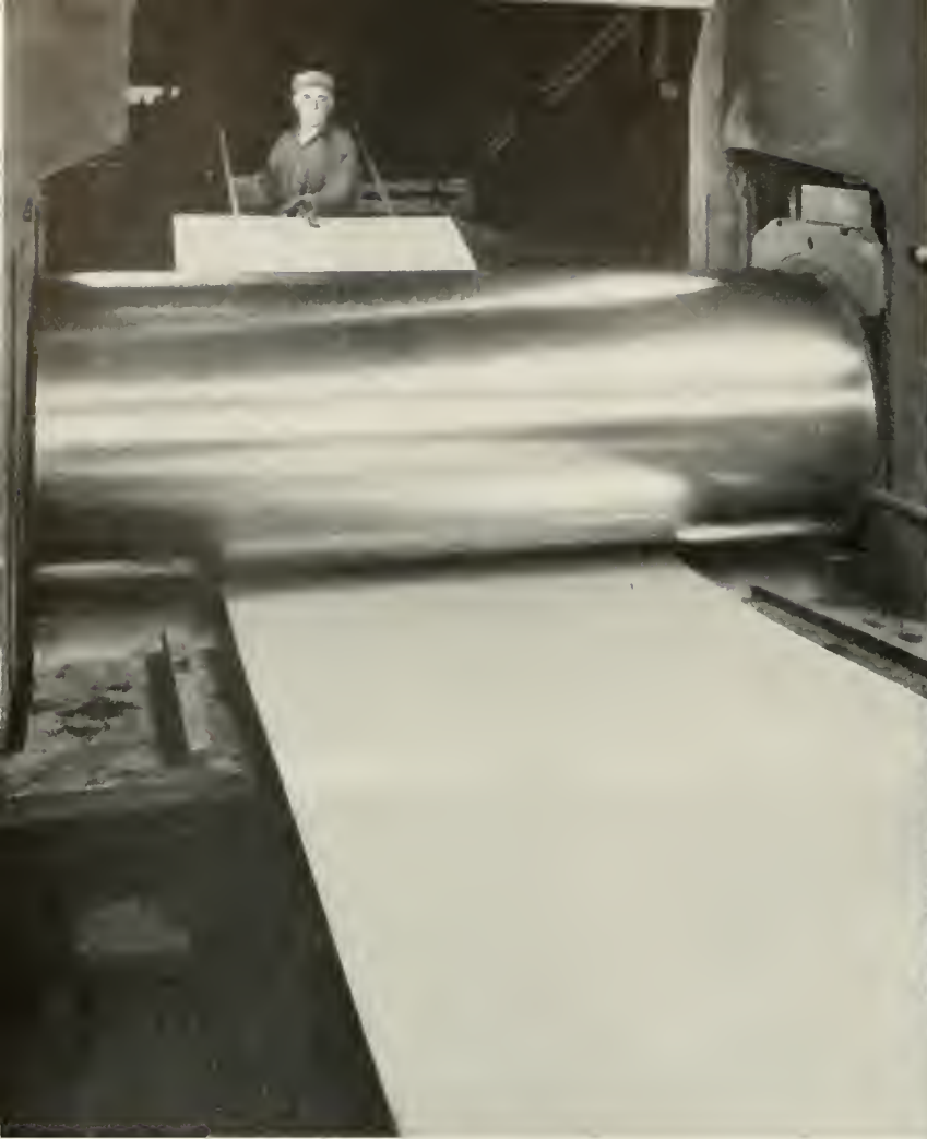
Fig. 6. (Above). Rolling stainless steel sheet at Wood Works, Carnegie-Illinois.
