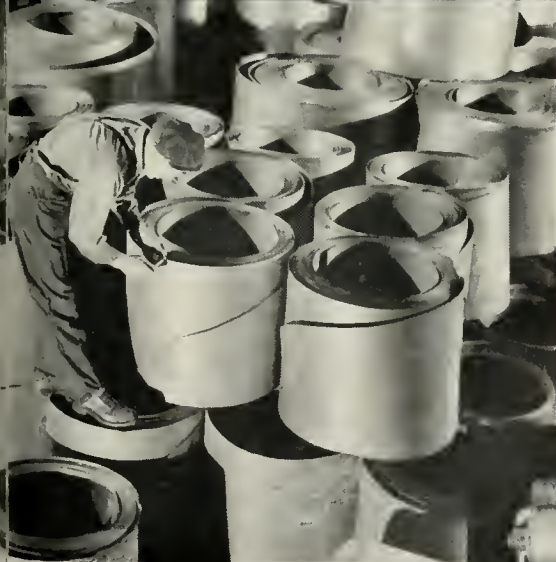
Fig. 4. (At left). Coils of hot-rolled stainless strip which will be further processed into cold-rolled strip or will be cut into breakdowns for rolling into sheets. The employee is putting a micrometer on the edges to see whether they are of the right thickness. This is called "inspecting for accuracy of gage." Gary Works, Carnegie-Illinois Steel Corpn., Gary, Ind.
