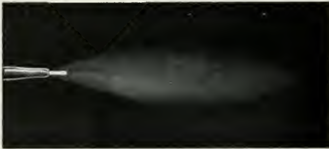
Fig. 1.—The neutral flame has an approximately one-to-one mixture of oxygen and acetylene
