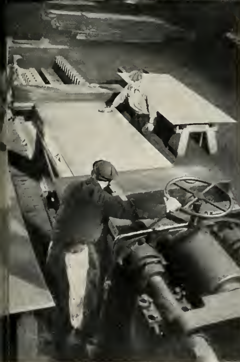
Fig. 13. (Right). Packing and crating stainless steel sheets, Wood Works. The polished sheets are interleaved with specially selected paper to prevent marring and scratching. The employee at the left is marking the sheet with a rubber stamp. Packing, inspecting and weighing are simultaneous operations here. The empty box and the paper are weighed first and the scale is set to tare. Hence when the box is packed the scale shows the net weight of the contents.
