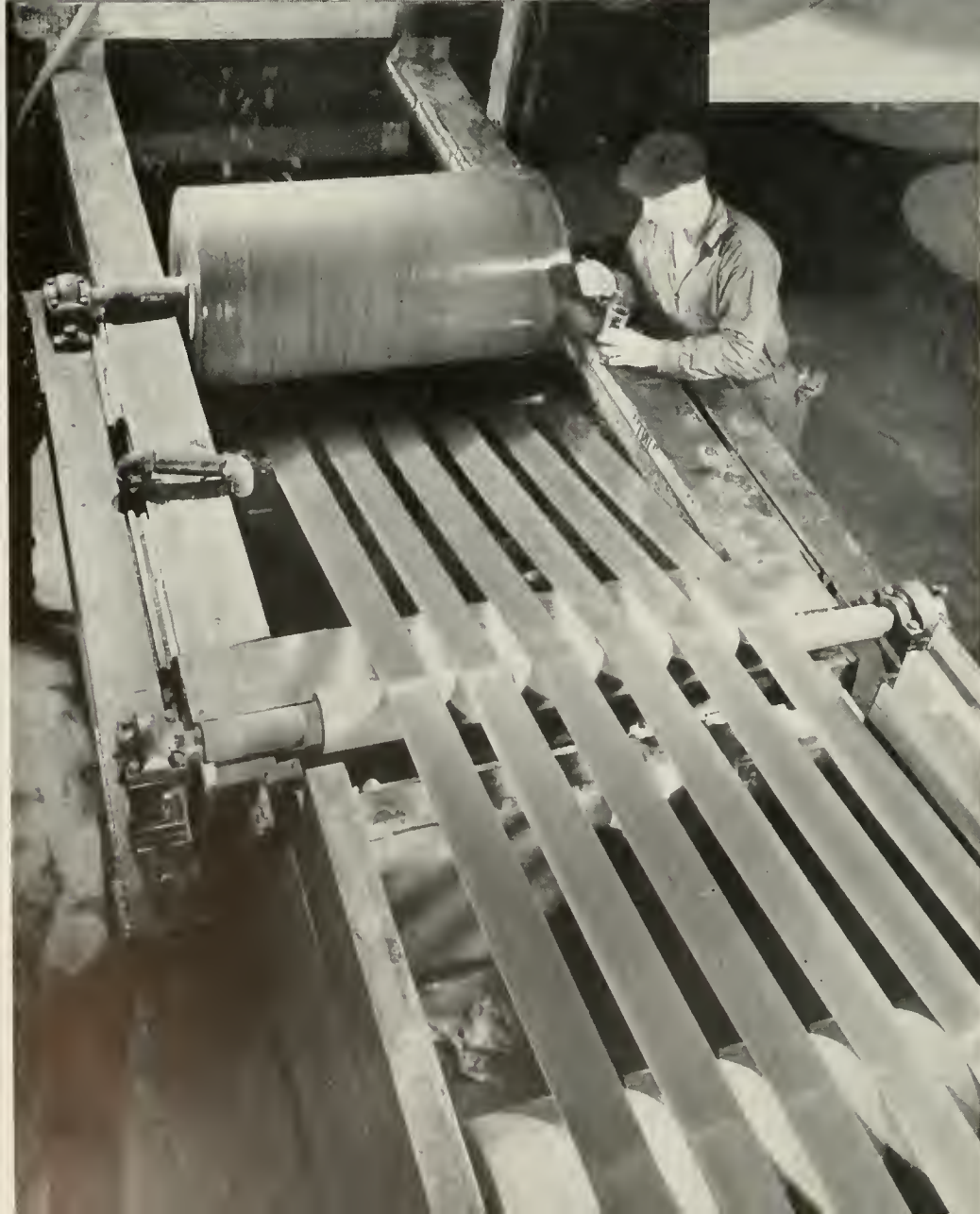
Fig. 16. (Left). Continuous pickling of cold-rolled stainless steel strip after annealing, Cuyahoga Works.
