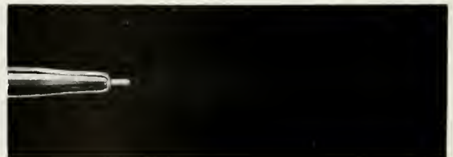
Fig. 3.—The oxidizing or excess oxygen flame is obtained by supplying additional oxygen to a neutral flame
