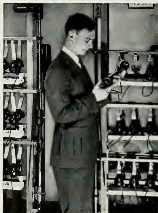
A Western Electric machine which puts telephones through their paces. Here representative samples receive a test which, in a few weeks, is equivalent to a lifetime of actual service.
