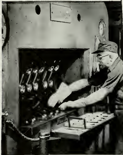
③ Moulding handles for telephone handsets—one of 248 parts in your Bell telephone.
