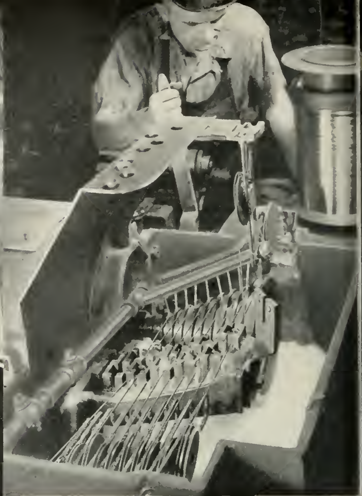
Fig. 22 (Above). Drawing extremely fine stainless steel wire, American Steel & Wire Co., Cleveland. Fig. 23. (Below). Annealing line stainless steel wire, American Steel & Wire Co., Cleveland.
