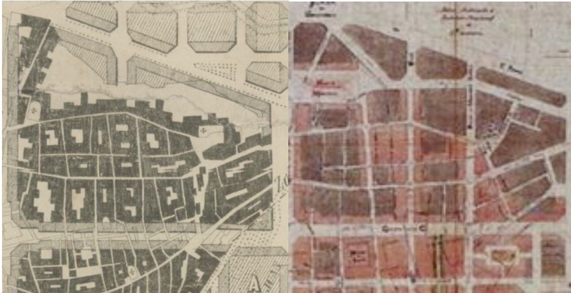
Fig. 5. 8: Comparative details of Cerdà's plan of urban reform (on the left) and Baixeras's proposal of reform (on the right). Notice how the irregular blocks of the old city are preserved in Cerdà's map—except for the opening of two of the three avenues included in his project—while Baixeras proposes to erase most of this section of the city in order to impose a quadrangular rationale that connects the old city with the Eixample.
