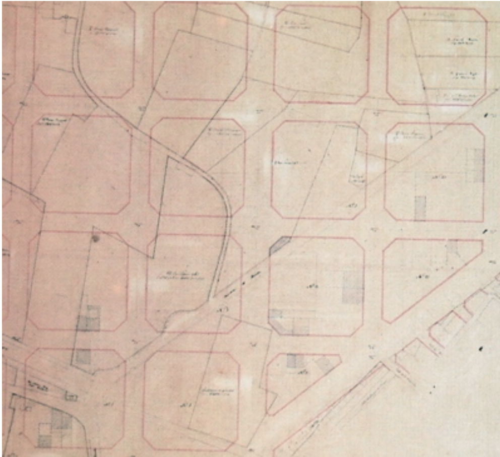
Fig. 3. 1: Detail of one of Cerdà's "planos particulares." Notice the imposition of the of the regular grid of the Eixample in red on top of the previous existing plots of the Barcelona plain in black. Ildefons Cerdà. "Plano particulario. Hoja XVI" 17 N/R 27 (Ref. 11224)" 1860-1865. 264 x 146 cm. Museu d'Història de la Ciutat de Barcelona.
