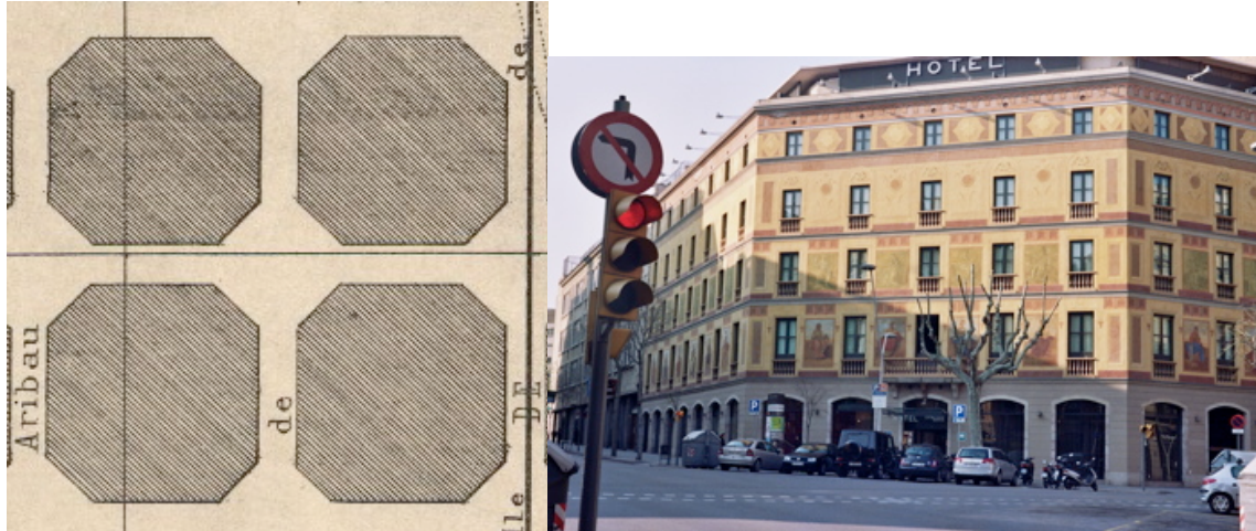
Fig. 4. 12: Basic layout of the blocs of the Eixample designed by Cerdà as they appear in Plano de Barcelona con la parte del Ensanche que se está edificando en la actualidad (1866) and a characteristic perspective of one of the first condominiums building of the Eixample in a photograph by Carlos Iglesias. This building was erected in 1862 at the confluence of Lluria and Consell de Cent streets.
