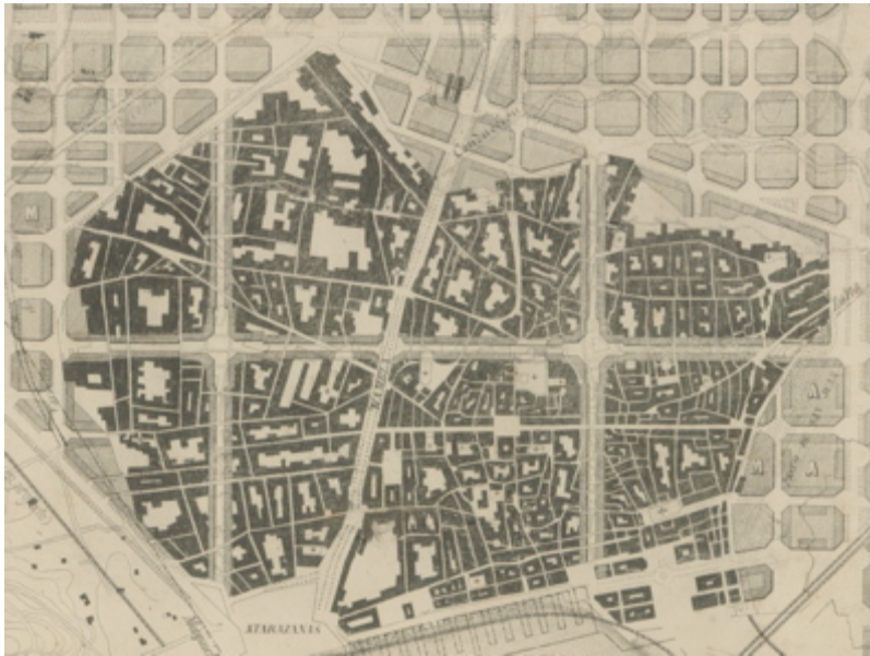
Fig. 5. 7: Baixeras plan of urban reform of the old city (up) contrasted with the comparatively limited span of Cerdà's proposal of reform (down). Baixeras modifies the layout of Cerdà's avenues A, B and C and introduces a comprehensive rationalization of the rest of the urban layout, especially on the northern section of the city, located on the right side of both maps.
