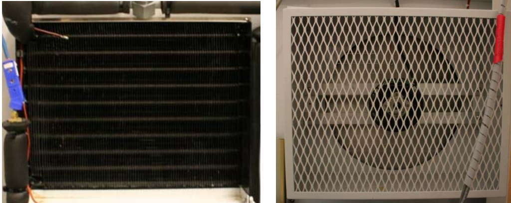
Figure 2.7 The condenser fan unit
