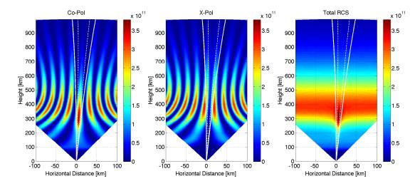
Figure 5.5 Co-polarized (left panel), cross-polarized (middle panel), and total (right panel) backscattered power detected by a pair of orthogonal linearly polarized antennas (see caption of Figure 5.4). Power levels are displayed in units of electron density. In each plot, the dashed white lines indicate the directions half a degree away from perpendicular to  $\mathbf{B}$ , while the continuous lines correspond to the directions one degree off.
