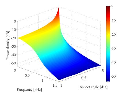
Figure 4.2 Simulated incoherent scatter spectra as a function of magnetic aspect angle and Doppler frequency for  $\lambda_B = 3 \text{ m}$  (e.g., Jicamarca radar Bragg wavelength). An O+ plasma with physical parameters given in Table 3.1 is considered.
