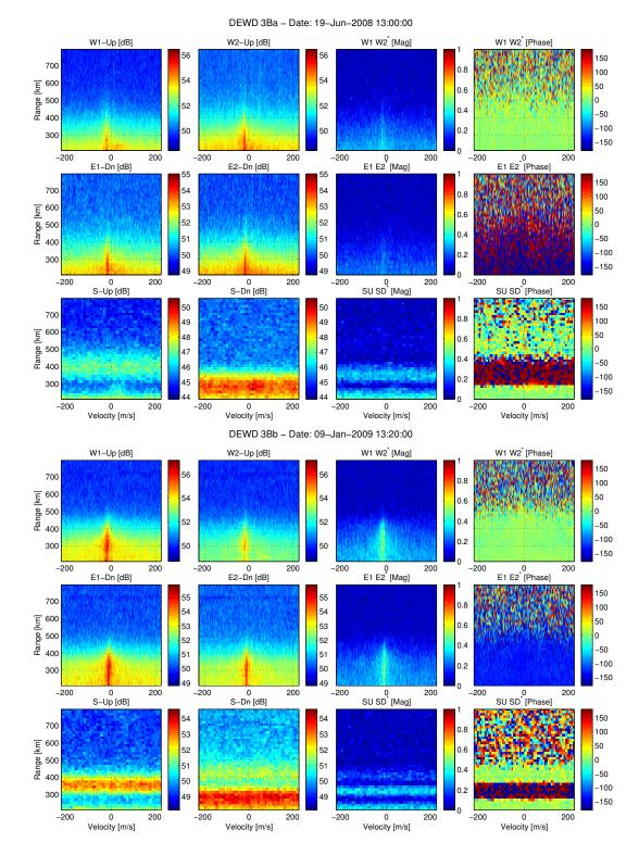
Figure 7.4 Sample self- and cross-spectra measured in the 3Ba experiment of June 19, 2008 (top rows), and in the 3Bb experiment of January 9, 2009 (bottom rows). The sample data were obtained after five minutes of integration. The self- and cross-spectra are plotted as functions of Doppler velocity and radar range.
