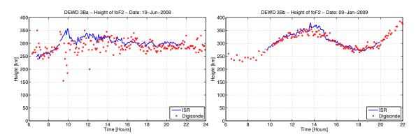
Figure 7.12 Comparison of the altitudes corresponding to the peak values of plasma frequency presented in Figure 7.11.
