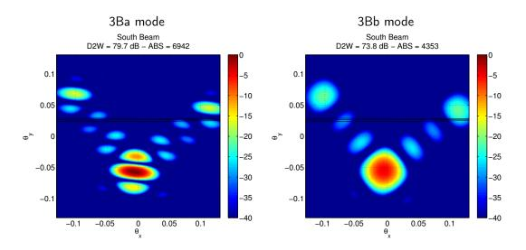
Figure 7.3 Two-way radiation patterns of the south beams used in the 3Ba (left) and 3Bb (right) experiments. Note that, in the north-south direction, the 3Ba south beam is narrower than the 3Bb beam.
