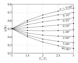
Figure 4.6 Electron scattering efficiency factor  $\eta(k)$  resulting from the frequency integration of the simulated incoherent scatter spectra as a function of electron-to-ion temperature ratio  $T_e/T_i$  and magnetic aspect angle  $\alpha$ . An O+ plasma with  $N_e = 10^{12} \text{ m}^{-3}$ ,  $T_i = 1000 \text{ K}$ , and  $B_o = 25 \,\mu\text{T}$  is considered.
