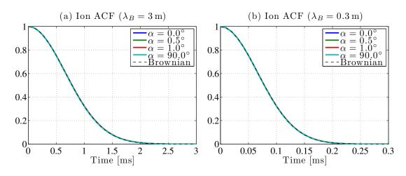
Figure 3.5 Simulated single-ion ACF's at different magnetic aspect angles  $\alpha$  for two radar Bragg wavelengths: (a)  $\lambda_B = 3 \text{ m}$  and (b)  $\lambda_B = 0.3 \text{ m}$ . The simulation results (color lines) are compared to theoretical ACF's computed using expression (3.22) of the Brownianmotion approximation (dashed lines). Note that there is effectively no dependence on aspect angle  $\alpha$ .
