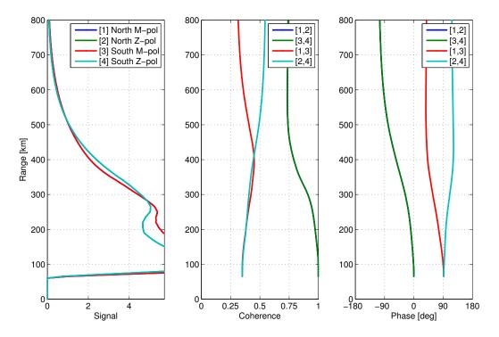
Figure 6.6 Simulated incoherent scatter signal power and coherence (magnitude and phase) profiles for the differential-phase radar configuration of June 8, 2004.
