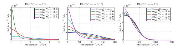
Figure 4.4 Electron density dependence of the simulated IS spectra for  $\lambda_B = 3 \text{ m}$  at aspect angles  $\alpha = 0^{\circ}$  (left panel),  $\alpha = 0.1^{\circ}$  (central panel), and  $\alpha = 1^{\circ}$  (right panel). An O+ plasma in thermal equilibrium with  $T_e = T_i = 1000 \text{ K}$  and  $B_o = 25 \,\mu\text{T}$  is considered. Note the different frequency scales used in each plot.
