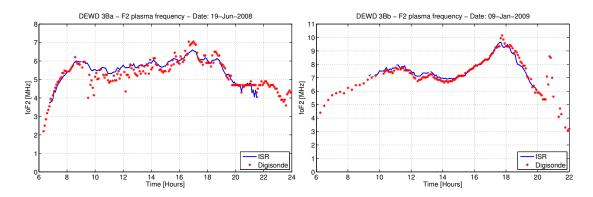
Figure 7.11 Comparison of the peak values of plasma frequencies (foF2) measured with the 3Ba and 3Bb radar techniques (blue lines) and with an ionosonde system also located at Jicamarca (red dots).
