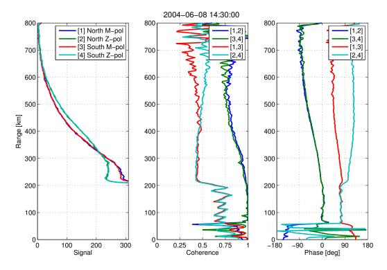
Figure 6.7 Measured incoherent scatter signal power and coherence (magnitude and phase) profiles that correspond to the differential-phase experiment conducted on June 8, 2004.
