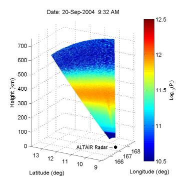
Figure 5.6 An example of the ALTAIR scan measurements collected during the 2004 EQUIS 2 campaign. In colors, levels of backscattered power calibrated to match electron densities in the probed region are displayed.
