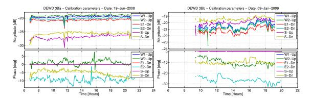
Figure 7.9 Magnitudes and phases of the radar calibration constants obtained as part of the inversion of the 3Ba and 3Bb radar data.
