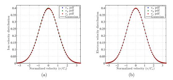
Figure 3.2 Probability distributions of (a) ion and (b) electron velocities resulting from the simulations. In each plot, the pdf's of the velocity components (displayed in colors) are compared to a Gaussian distribution (black line). Notice that the velocity axes are normalized by the thermal speeds of the corresponding particle species. The plasma parameters considered in the simulations are given in Table 3.1.
