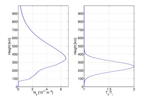
Figure 5.3 Electron density and  $T_e/T_i$  profiles as functions of height.
