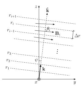
Figure 5.2 Geometry of wave propagation in an inhomogeneous magnetized ionosphere.
