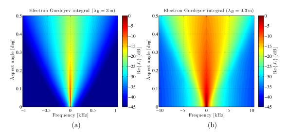
Figure 4.1 Simulated electron Gordeyev integrals as functions of Doppler frequency and magnetic aspect angle for two radar Bragg wavelengths: (a)  $\lambda_B = 3 \text{ m}$  and (b)  $\lambda_B = 0.3 \text{ m}$ . An O+ plasma with electron density  $N_e = 10^{12} \text{ m}^{-3}$ , temperatures  $T_e = T_i = 1000 \text{ K}$ , and magnetic field  $B_o = 25 \,\mu\text{T}$  is considered.
