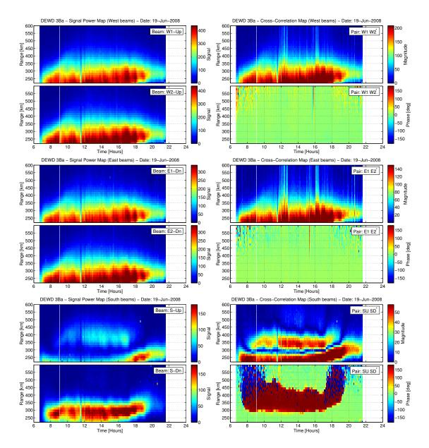
Figure 7.5 Range vs. time plots of the signal power and cross-correlation data measured in the 3Ba experiment of June 19, 2008. On the left, the power data collected by each of the radar beams are displayed in linear scale. On the right, the magnitudes of the cross-correlation data are also plotted in linear scale, while the phase data are plotted in degrees.
