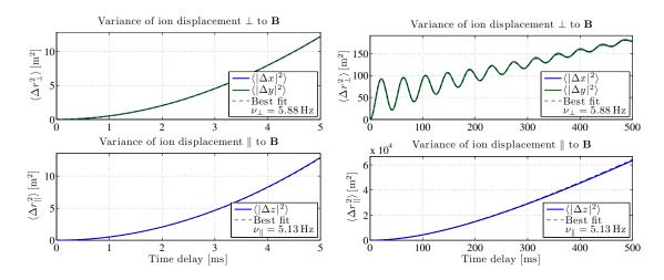
Figure 3.4 Variances of the displacements of a simulated ion in the directions perpendicular (top panels) and parallel (bottom panels) to the magnetic field. The simulation results (color lines) are displayed for two time intervals: 5 ms (left panels) and 500 ms (right panels). The dashed lines correspond to the fits of the results to the theoretical expressions for  $\langle \Delta r_{\perp}^2 \rangle$  and  $\langle \Delta r_{\parallel}^2 \rangle$  of the Brownian-motion model.
