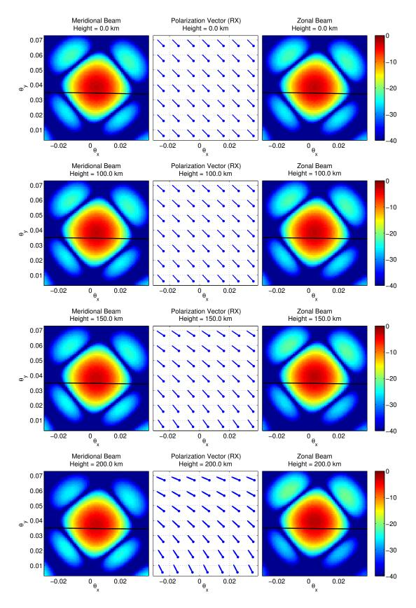
Figure 6.3 Meridional and zonal effective radiation patterns for r = 0, 100, 150, 200 km.
