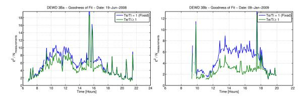
Figure 7.10 Goodness-of-fit values resulting from the inversion of the 3Ba and 3Bb radar data. The blue curves correspond to the values obtained by fitting only for the electron density  $N_e$  and assuming that  $T_e/T_i = 1$  at all altitudes. The green curves correspond to the values obtained by fitting for both parameters,  $N_e$  and  $T_e/T_i$ .
