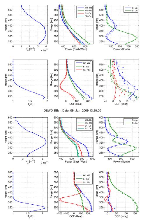
Figure 7.7 Sample plots of the results obtained from the inversion of the 3Ba and 3Bb data (top and bottom panels, respectively). The estimated  $N_e$  and  $T_e/T_i$  profiles are plotted in the left column. In the other columns, the power and cross-correlation measurements (dotted points) are compared with the modeled profiles (continuous lines).
