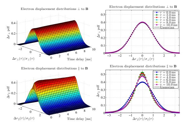
Figure 3.6 Same as Figure 3.3 but for the case of a simulated electron. All distributions at all time delays are normalized to unit variance. Note that the distributions of the displacements parallel to  $\mathbf{B}$  become narrower than a Gaussian distribution in less than a millisecond.
