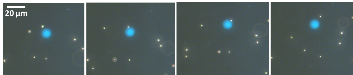
Figure 6.8 A time sequence of 4 dark field optical images showing a gold particle with local negative approaches a phosphate giant vesicle and detaches from it.
