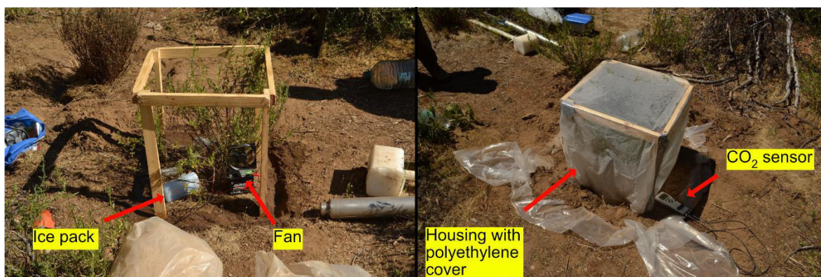
Figure 1.2.2: Field labeling setup. The labeling chamber was constructed as a wooden frame around the investigated specimens which were covered by polyethylene foil for the labeling. An ice pack and fan were placed in the labeling chamber to keep temperatures inside at ambient level. The \text{CO}_2 concentration in the labeling chamber was monitored with a \text{CO}_2 sensor.
