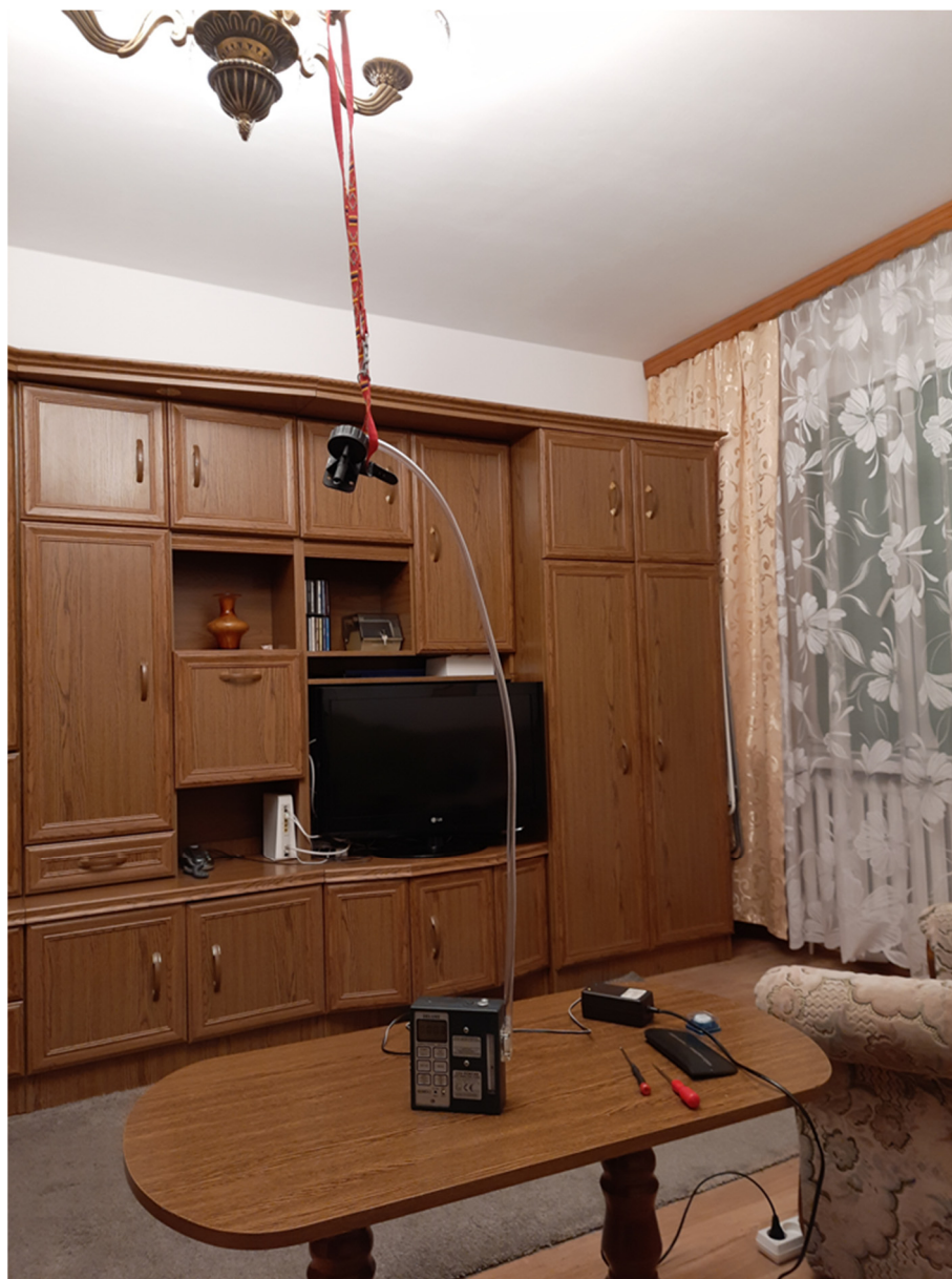
Figure 2. Photo of the SKC sampler with a head equipped with a cyclone with a cut-off diameter of 4\ \mu\text{m} while measuring the concentration of airborne particles in one of the reference apartments in Katowice (no smokers).
