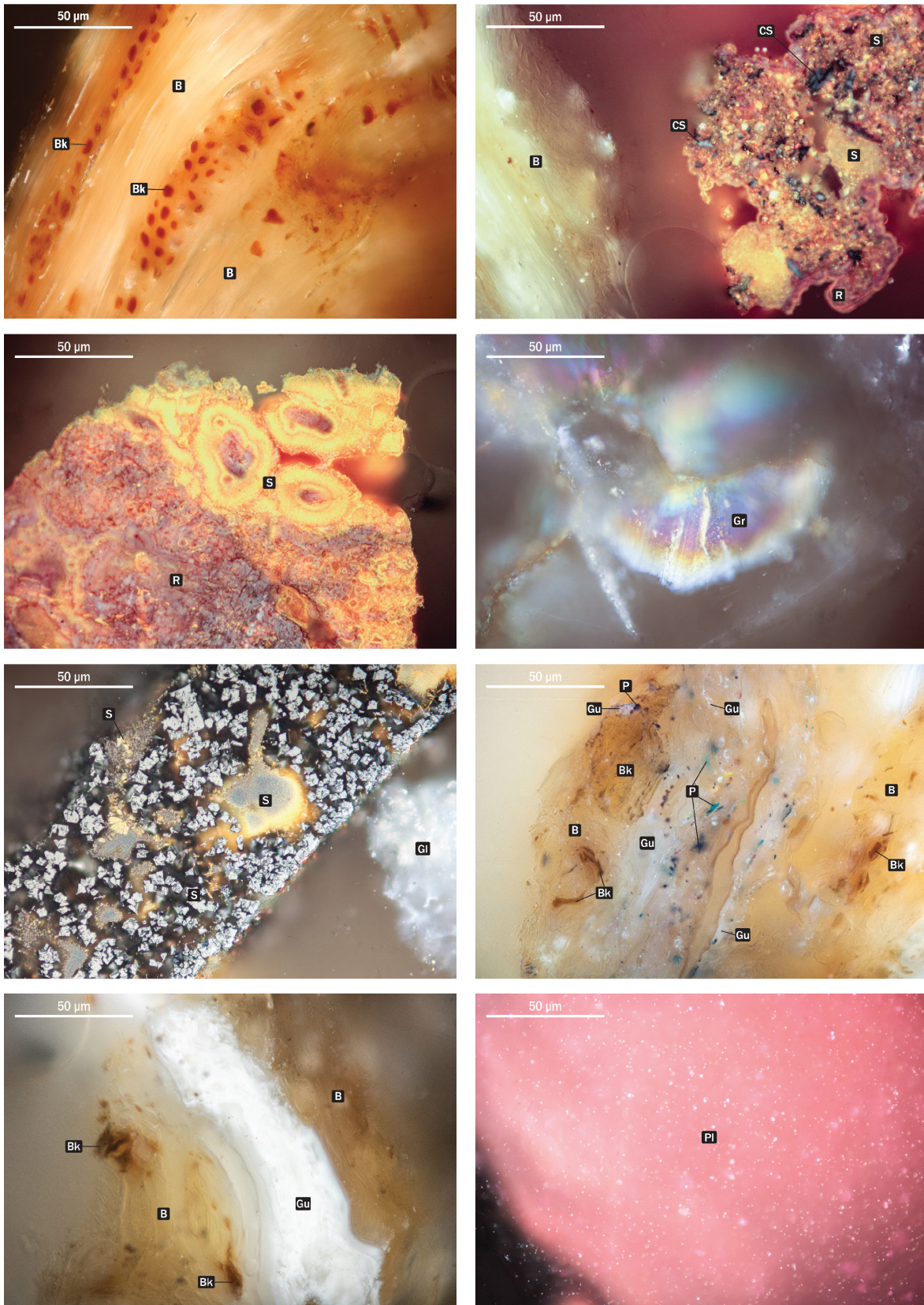
Figure 2. Photomicrographs of selected wood pellet components in reflected white light and oil immersion. B = biomass, Bk = bark, CS = coal in slag, Gl = glass, Gr = grease, Gu = glue, P = paint, Pl = plastic S = slag, R = rust.
