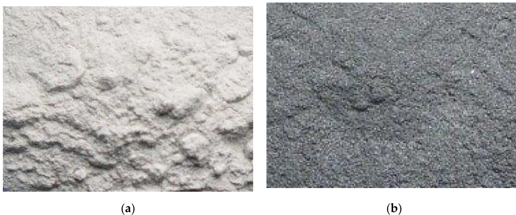
Figure 2. ZrO_2 obtained as a sludge during leaching of waste from the plasma treatment of metal surfaces (a) and Ni–P– ZrO_2 composite powder after the electrodeposition process (b).
