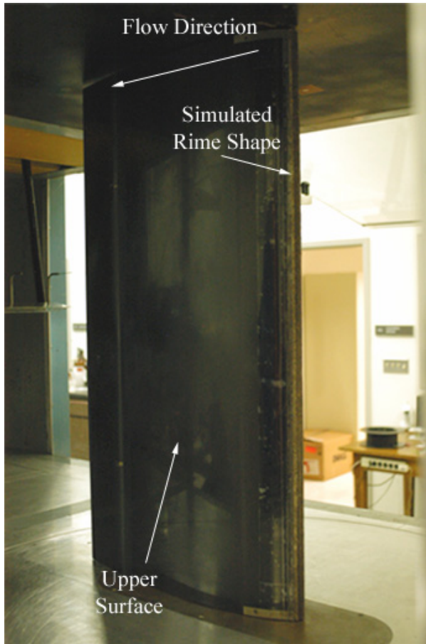
Fig. 2.17 Simulated rime ice on NACA 3415 model, a) full view; b) detail view.
