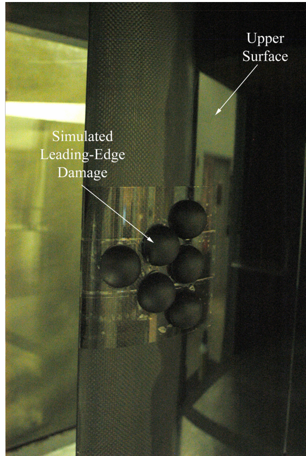
Fig. 2.25 Simulated leading-edge damage on NACA 23012 model, a) full view; b) detail view.
