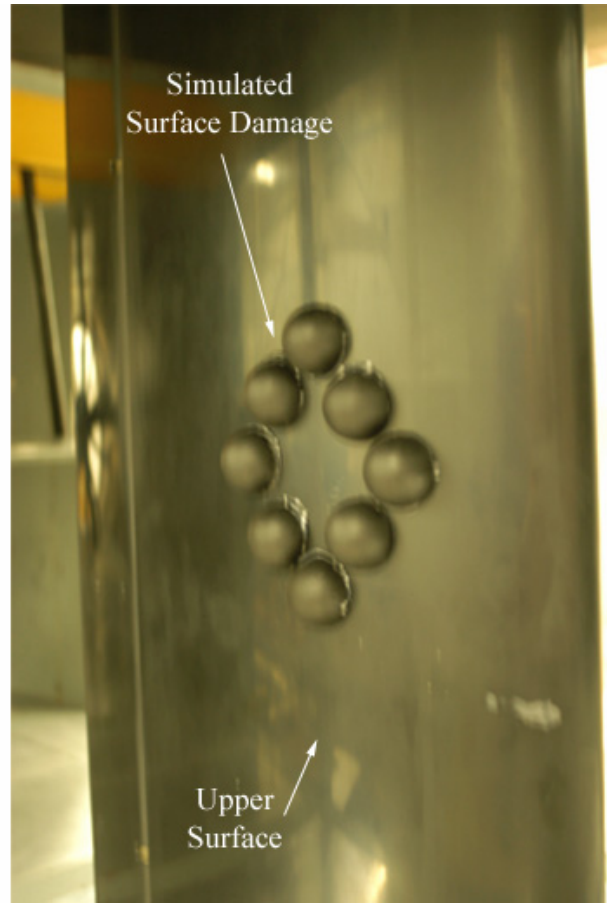
Fig. 2.26 Simulated upper-surface damage on NACA 3415 model, a) full view; b) detail view.
