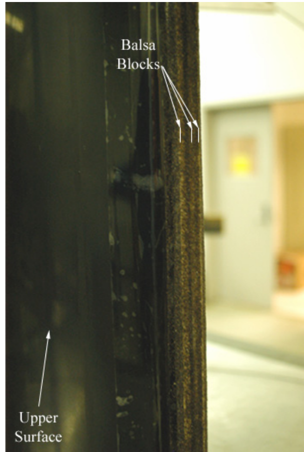
Fig. 2.17 Simulated rime ice on NACA 3415 model, a) full view; b) detail view.
