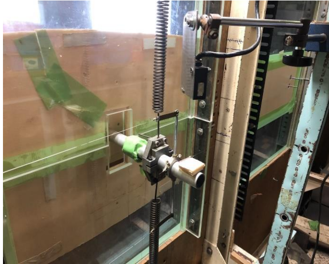
Figure 6.1.8 Suspension situation outside the wind tunnel
