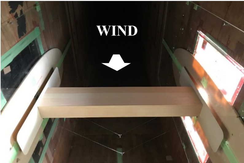
Figure 4.1.1 Sectional model of B/D=2.0 in the wind tunnel
