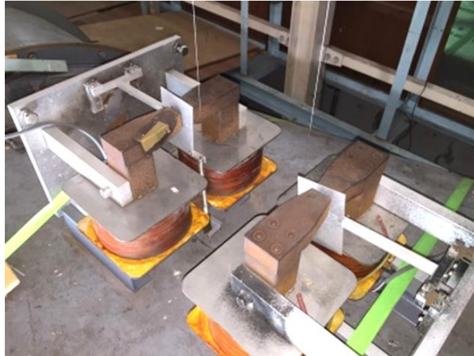
Figure 3.1.4 Setting situation of the magnetic dampers
