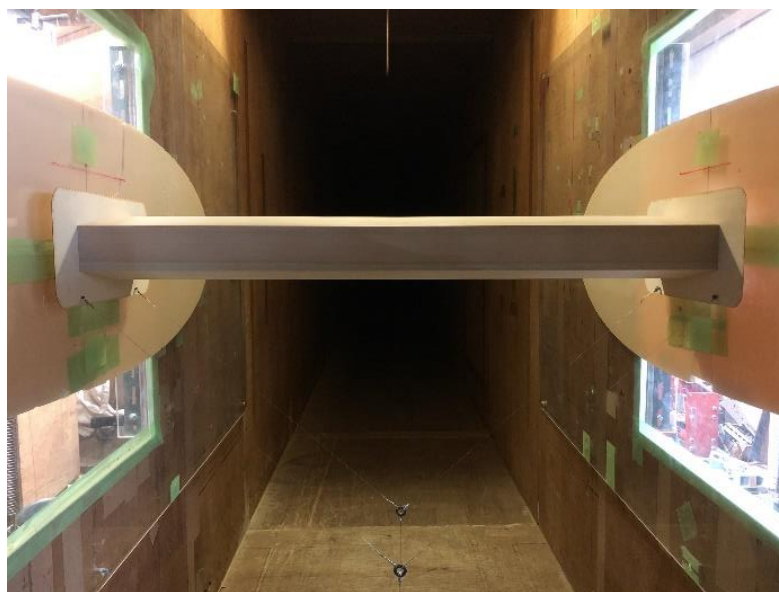
Figure 6.1.5 Sectional model of TYPE-1 cross section ( \theta=10^\circ ) inside the wind tunnel
