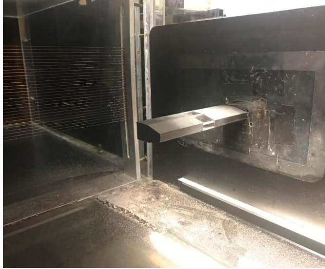
Figure 6.1.11 Setting situation of the model of TYPE-1( \theta=15^\circ ) inside the wind tunnel
