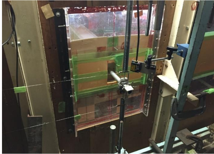
Figure 4.1.4 Suspension situation outside the wind tunnel
