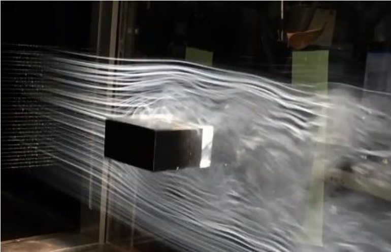
Figure 5.1.4 Forced-oscillating model of B/D=2.0 in the wind tunnel
