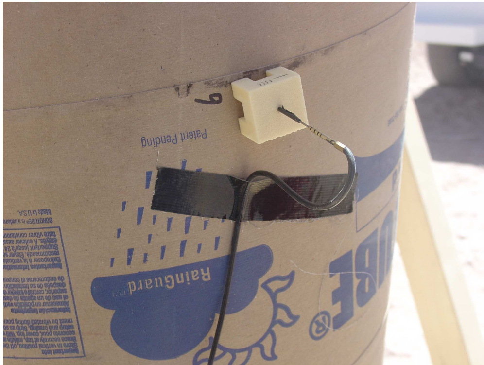
Figure 6.1: Shorting pin mounted in an assembled charge to record the detonation velocity.
