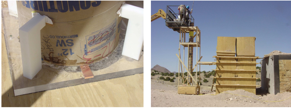
(a) Plexiglas plate mounted to the bottom of the cardboard confiner of a charge. (b) An assembled 304.8 mm charge during the filling operation.
