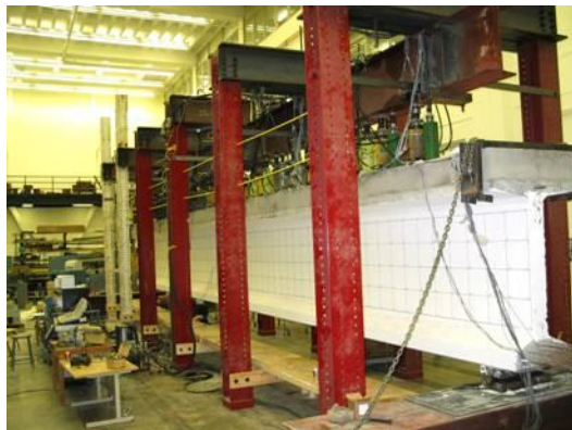
(a) Girder in test setup
