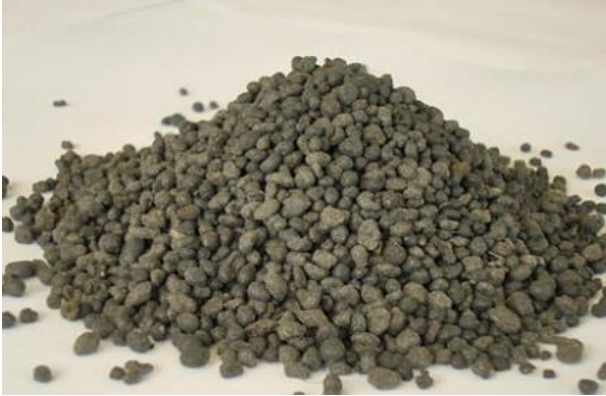
Figure 3.11 – The general view of the organo-mineral composite material based on phosphogypsum and sewage sludge after the anaerobic stabilization under conditions of dissimilating sulfate reduction (in the biocomposite)
