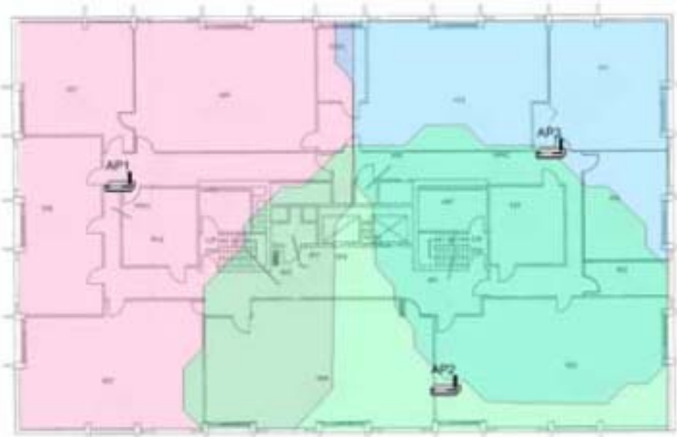
Figure 3. Signal on 4 th floor from 4 th floor
