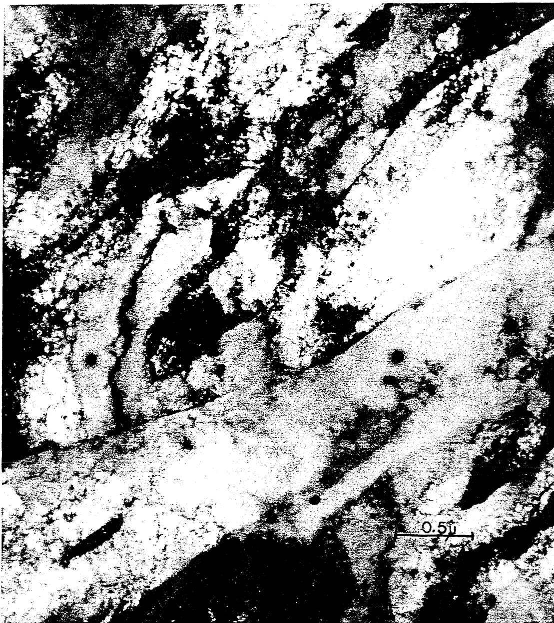
FIG. II TRANSMISSION ELECTRON MICROGRAPH OF THE SOLUTION TREATED 12% NICKEL MARAGING STEEL
