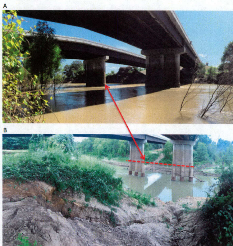
Figure 2. Trinity sampling site near Oakwood (station 3) during July 2015 when discharge was 17,000 cfs (A) and June 2018 when discharge was 850 cfs (B). A common point of reference between the two sampling years (double-headed arrow line) and the high-water discharge height (dashed line) are shown.
