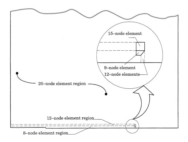
Figure 8. Distribution of finite elements (2 layers through thickness everywhere)
