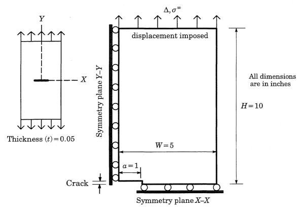
Figure 1. Quarter symmetric geometry of M(T) plate
