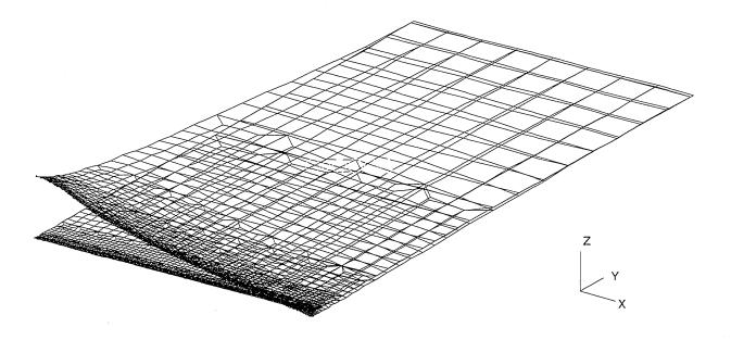
$\textbf{Figure 5.} \ \textbf{Deformed shape nonlinear analysis (shell elements)}$
