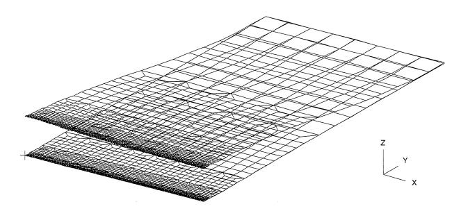
Figure 4. Deformed shape for linear analysis (shell elements)
