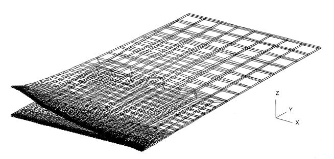
Figure 6. Deformed shape for nonlinear analysis (solid elements)
