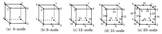
Figure 7. Warp3D solid elements
