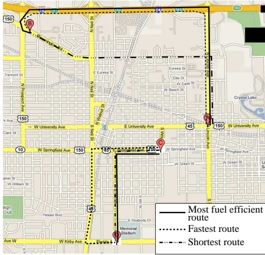
(a) Figure showing the driving routes used in Experiment 1 (from point A to point B) and Experiment 2 (from point C to point D). Routes with dashed and dotted lines are shortest-path routes while routes with dash lines are fastest routes provided from MapQuest system. The most fuel efficient route is marked by solid lines. Experiment 1 was conducted using a Honda Civic, 2002 and Experiment 2 using a Pontiac Grand AM, 1997.
