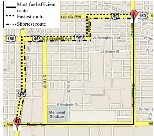
(b) Figure showing the example of the most fuel-efficient route that is different from the fastest and shortest-path route. The route with solid lines is the fastest and shortest-path route from point A to point B provided by MapQuest system. The route with dash lines is the most fuel-efficient route. The car used for collecting data was a Pontiac Grand AM, 1997.
