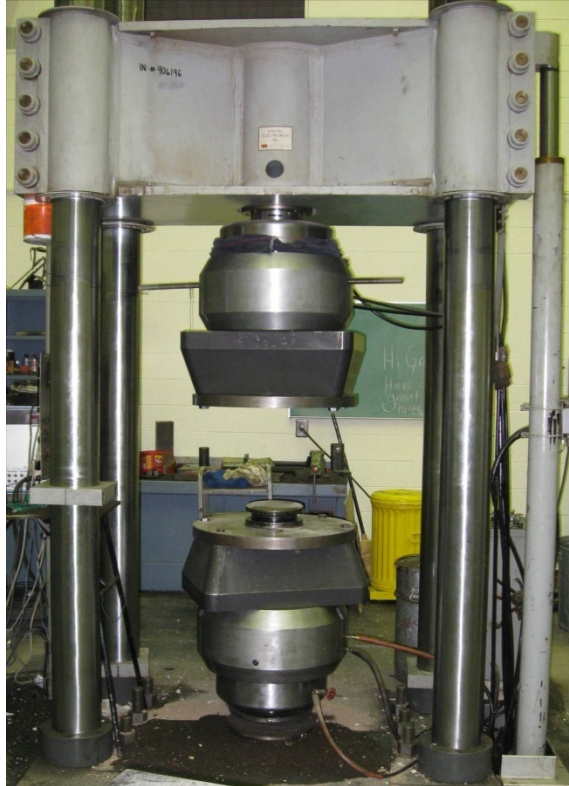
Figure 13. 600 kip MTS testing machine.
