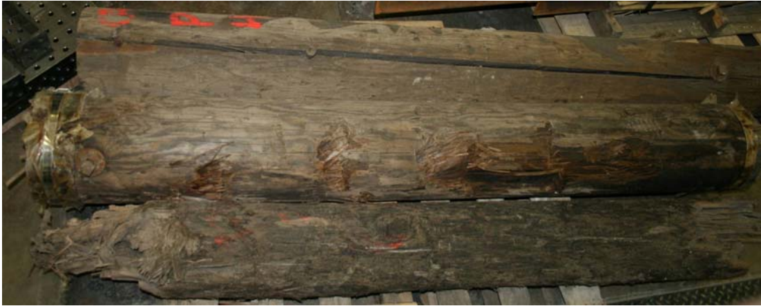
Figure 8. Retrieved pile samples.
