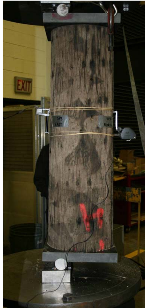
Figure 25. Loading end plate in testing frame.
