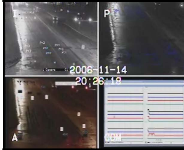
Figure 3.8. Sample image of missed call in Zone 6 due to reflection of headlights.
