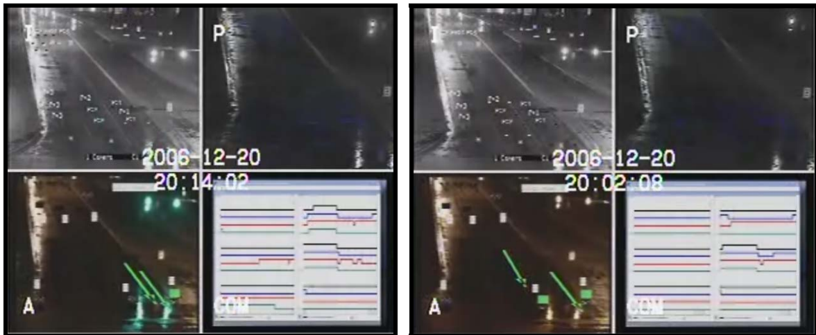
Figure 3.6. Sample images of false calls in stop bar zones due to reflection of traffic lights.
