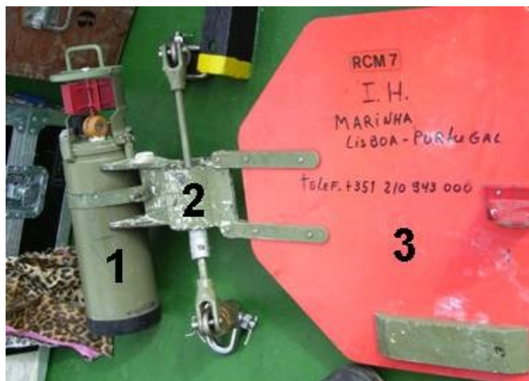
Figure 4 – Aanderaa RCM7 current meter The Aanderaa RCM7 current meter consists of three fundamental components: the pressure box (1), the rudder body (2) and the rudder plate (3)
