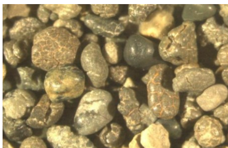
Figure 5.29 - Fractures along glauconitic grains.
