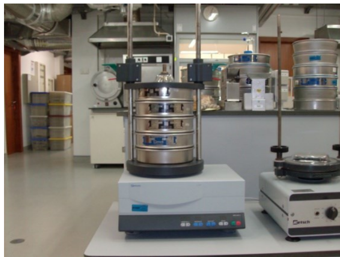
Figure 10 - Sieving equipment with 0.5 phi interval.
