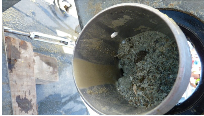
Figure 2 - Sediment core collect at Ericeira mud patch in N.R.P. “Auriga”.
