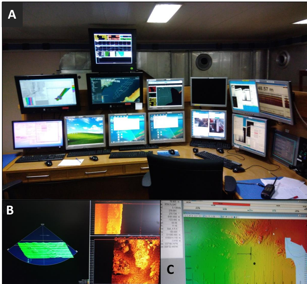
FIGURE 4.6 – (A) - Bathymetry survey room on the RV Sarmiento de Gamboa. (B) – Example of an acquisition panel in a campaign. (C) – Seafloor bathymetry covering map.
