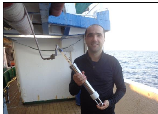
FIGURE 4.7 – Sound velocity profiler (SVP), before measuring the sound velocity in the water.
