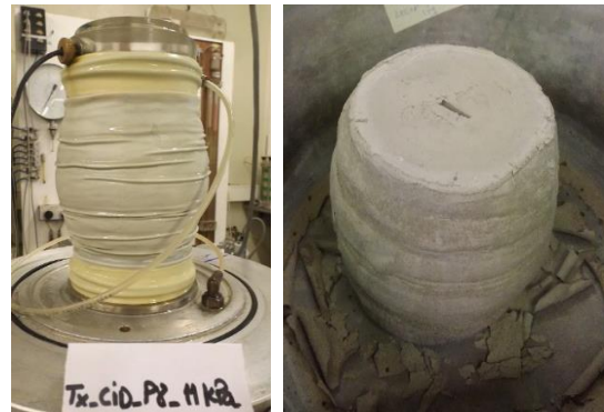
FIGURE 7.20 – Barrel-shaped disrupted specimen after triaxial compression.
