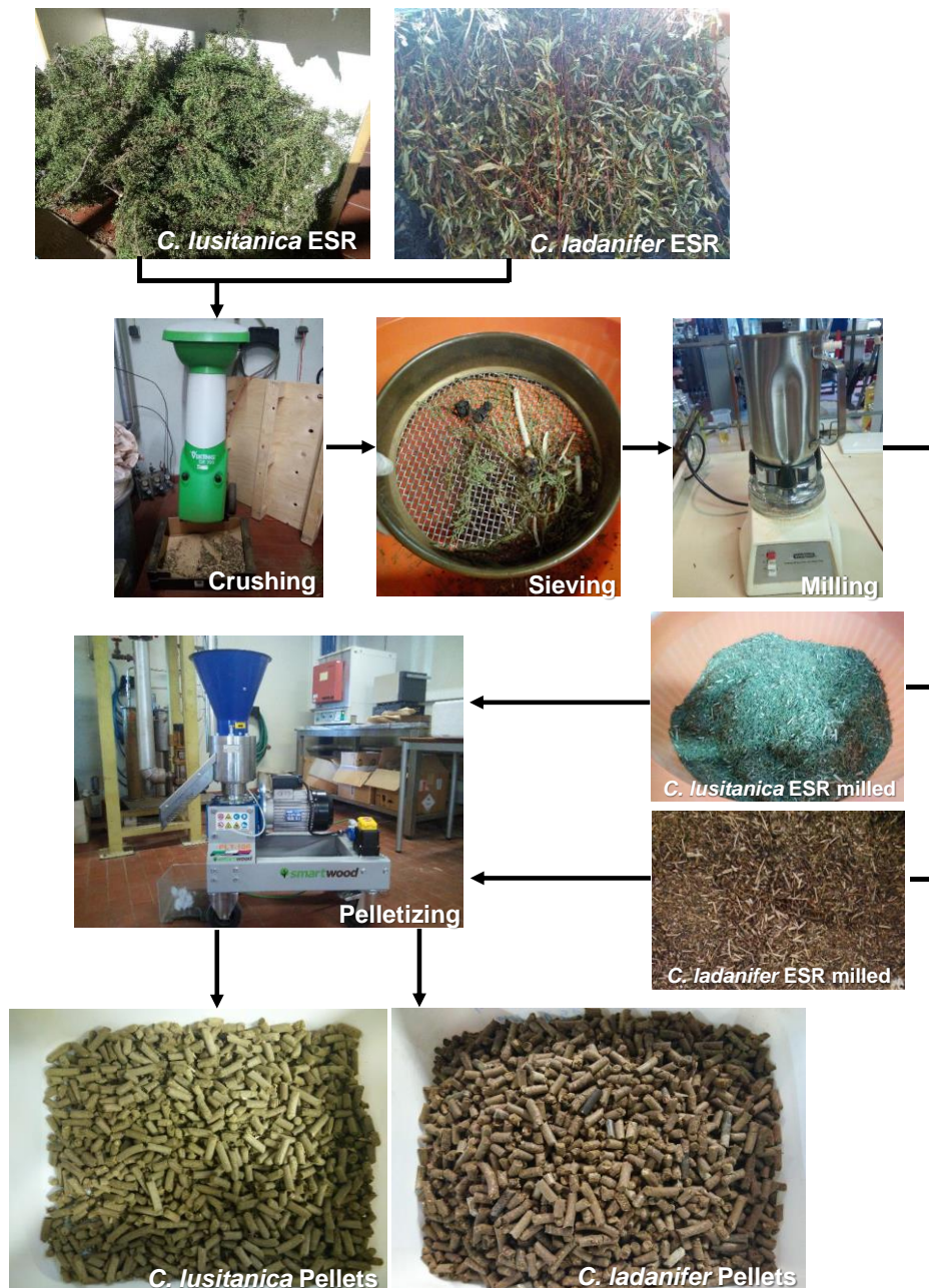
Figure 4.1. Flowchart for pellets production from C. lusitanica and C. ladanifer .
