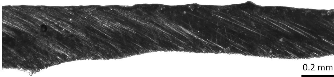
Figure 3.13 - Cross section view of a ribbon, grown with a [75; 106] \mu\text{m} particle size powder substrate, obtained by mechanical polishing a recrystallized area.
