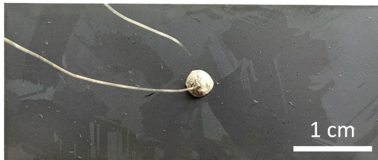
Figure 2.12 - Type-K thermocouple glued to the back surface of a multicrystalline silicon substrate.
