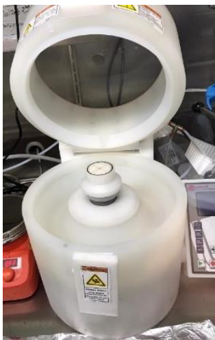
Figure 2.13. Picture of the spin coater which is used for depositing active layers in PSCs
