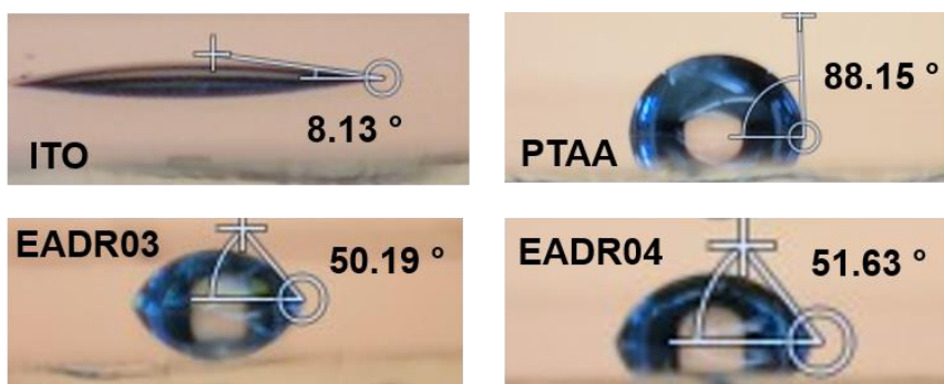
Figure 5.4. Contact angle measurements on the bare ITO, ITO/PTAA, ITO/EADRo 3 and ITO/EADRo 4 surfaces.
