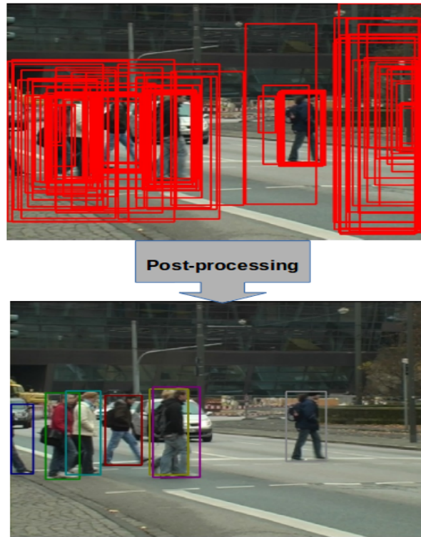
Figure 2.1: Detection proposals to final bounding boxes: for object detection, on the top, (100) detection proposals (generated by Faster-RCNN) detector, will pass through a post-processing step (GreedyNMS is used by default), and acquire the final bounding boxes as shown at the bottom.
