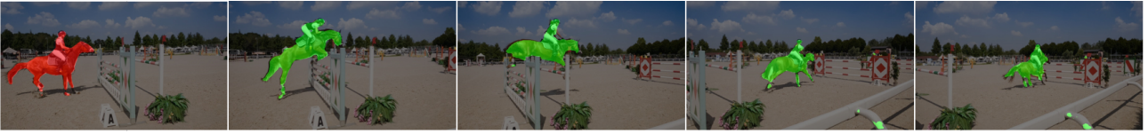
Figure 2.3: Video object segmentation: The per-pixel dense annotation of the first frame (red) is given, the goal for video object segmentation is to acquire the segmentation mask in the rest of the frames independently (green).
