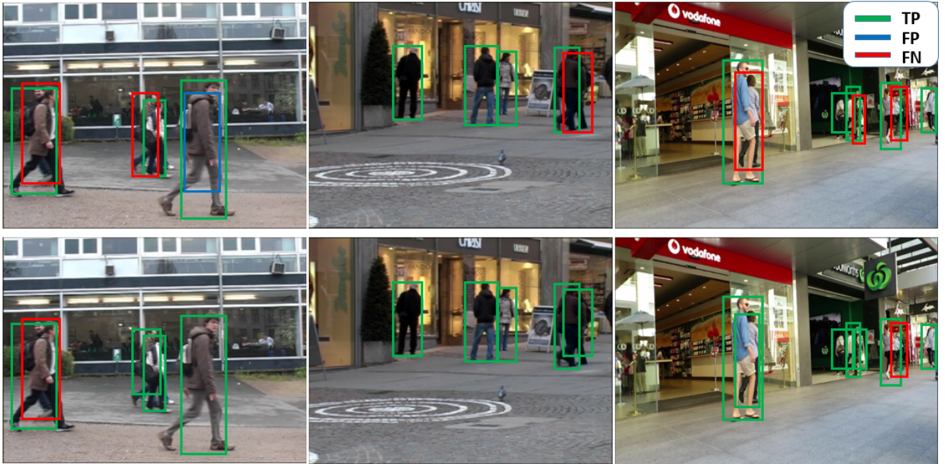
Figure 3.9: Visualized detections of GreedyNMS (the first row) and Pairwise-NMS (the second row). With green box, blue box, and red box to denote true positive, false positive and false negative, respectively. As can be seen, compared with the detection results acquired from GreedyNMS, the detection results acquired from Pairwise-NMS dramatically reduce the false negatives (which leads to the higher recall), and meanwhile reduce the false positives slightly (which contributes to the precision).
