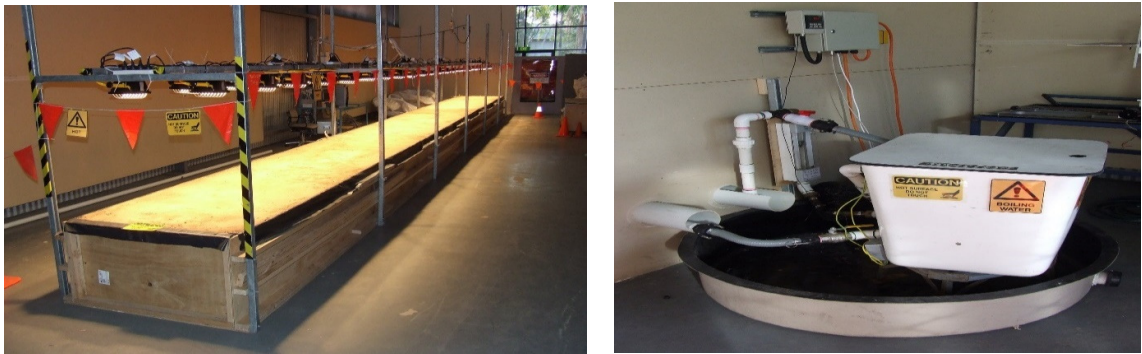
Figure 4.8: Photographs of the experimental set up. Sandy loam bed and lamps (left) and water heating system (right)
